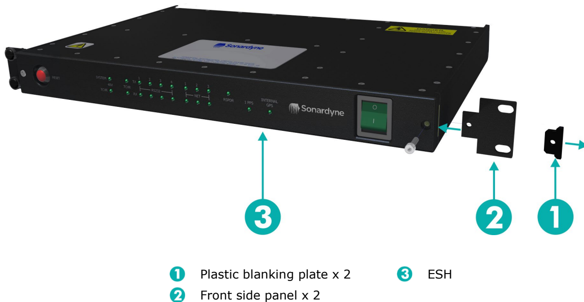
Figure 4-1 Front rack mounting side panel installation
