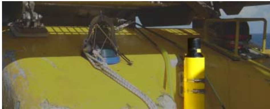
Fig 60 Inappropriate beacon mounting
