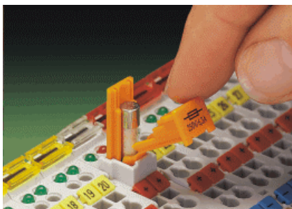
Fig. 1.6: Opening the fuse holder
