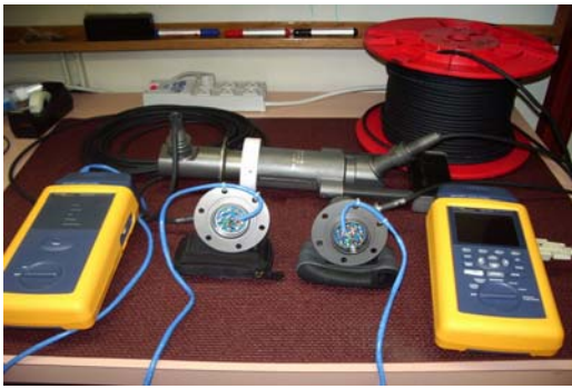
Fig 2: Test setup at WHOI. Ethernet channel consisting of a penetrator, 10meter Cat5e cable, ODI underwater ROV wet-mateable connector, 90 meters Cat5e cable, and a second penetrator. Physical Ethernet characteristic tests are conducted with Fluke DSP4000 series cable analyzer.
