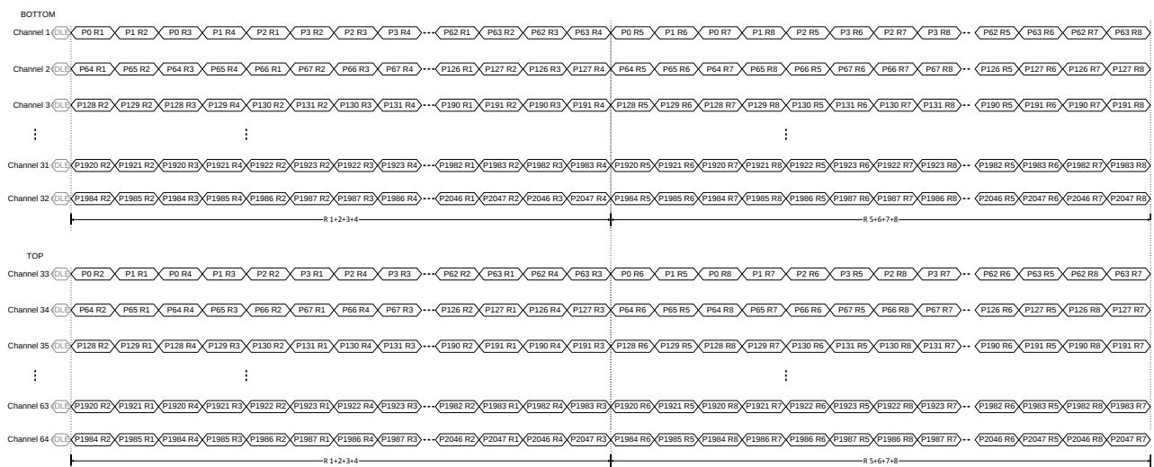
FIGURE 53: COLOR BINNING, PIXEL TO OUTPUT REMAPPING
