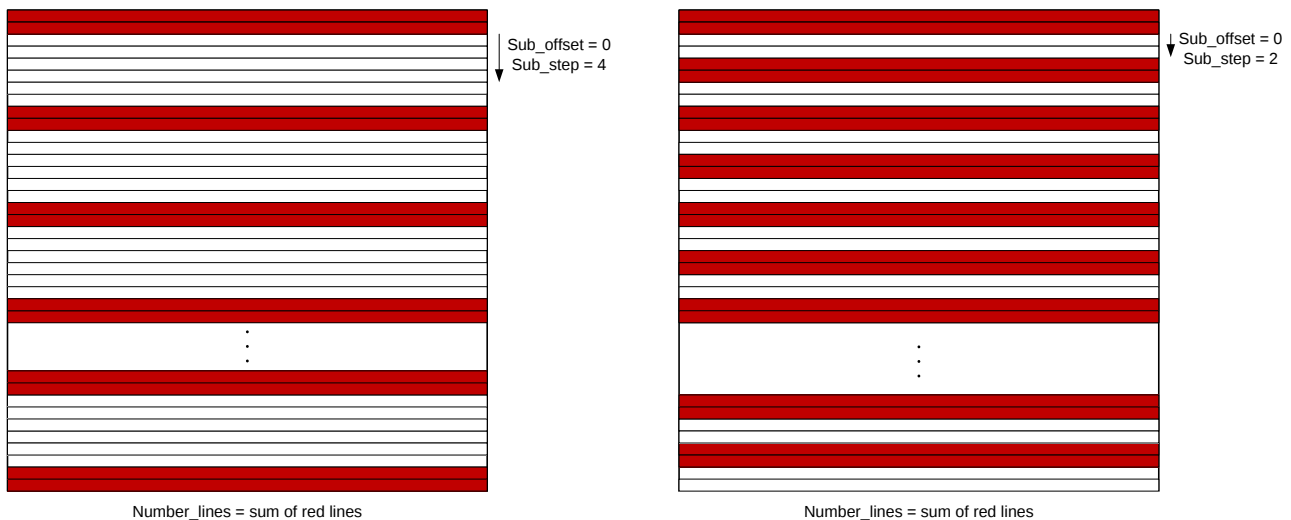
FIGURE 46: SUBSAMPLING IN Y EXAMPLES IN COLOR MODE (SKIP 6X AND SKIP2X)
