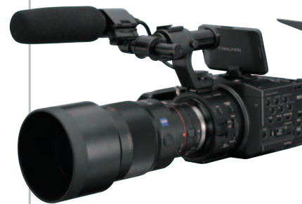
A-mount lens with the LA-EA1 adaptor
