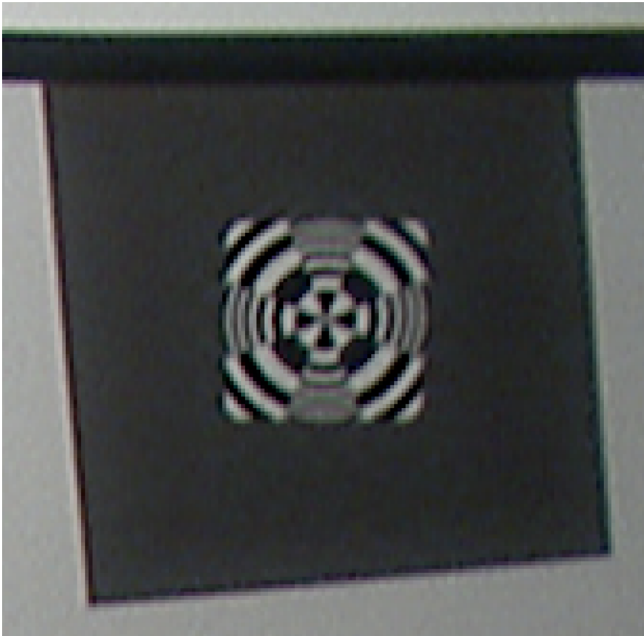
Sony HDCP1, Zeiss 5mm Lens, 160 lux, 85 IRE, Target 38 inches, detail ON (25) File: Test_90.tiff
