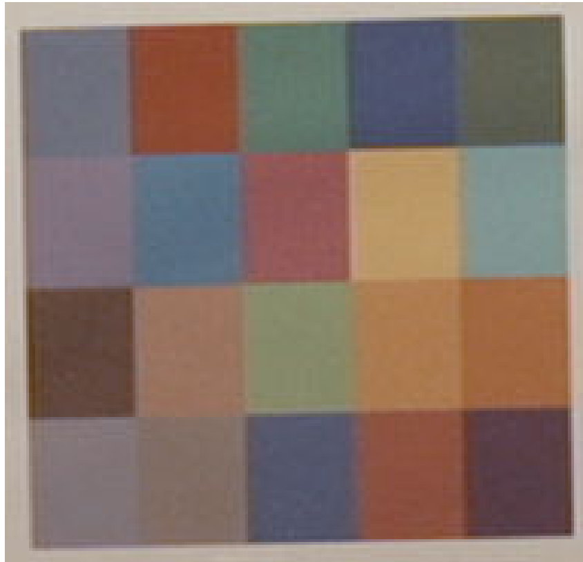
Sony NEX-FS700U, Sony 11mm Lens, 150 lux, ISO 2000, Target 38 inches (w/mild color correction)
