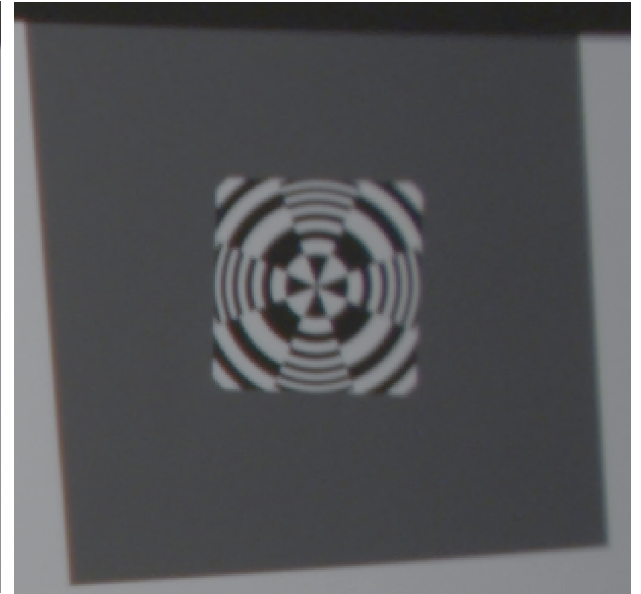
Sony F-5, Zeiss 12mm T2.1 Standard Prime Lens, 800 lux, EI 2000, Target 34 inches, 4K P60 File: Test_54B_4K_DPX.tiff
