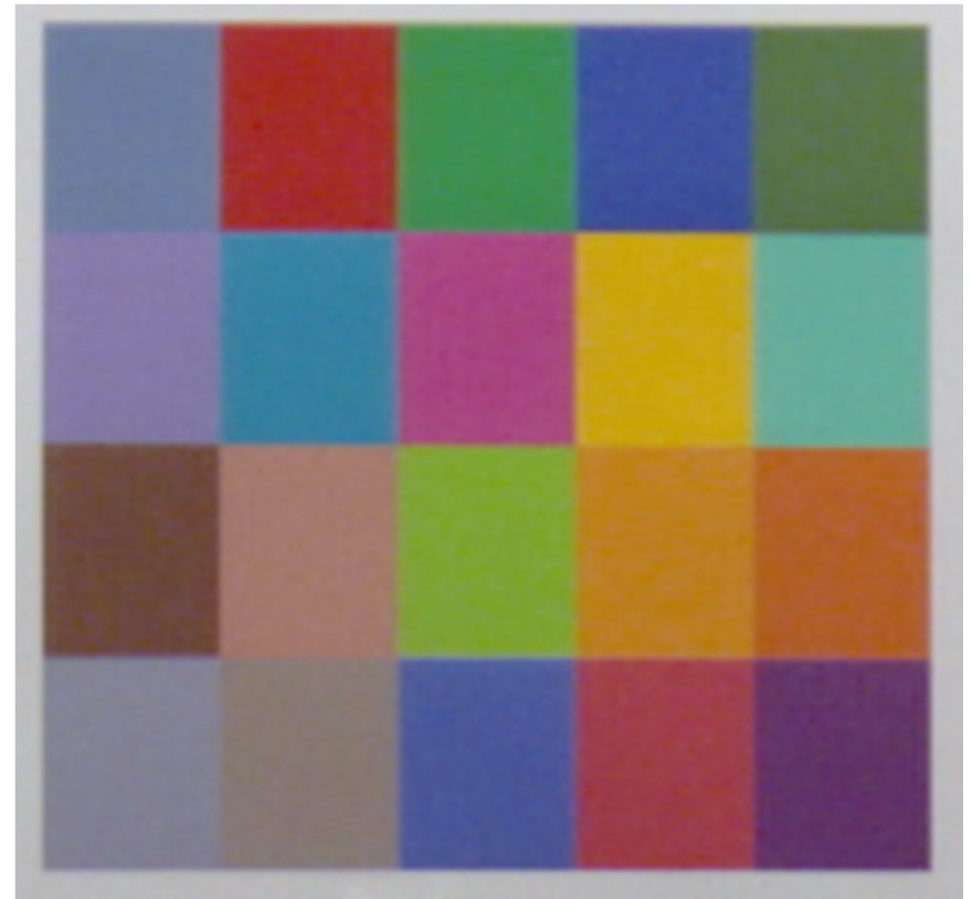
Ikegami HDL-50/HS, Zeiss 5mm Lens, 140 lux, 80 IRE, Target 38 inches
