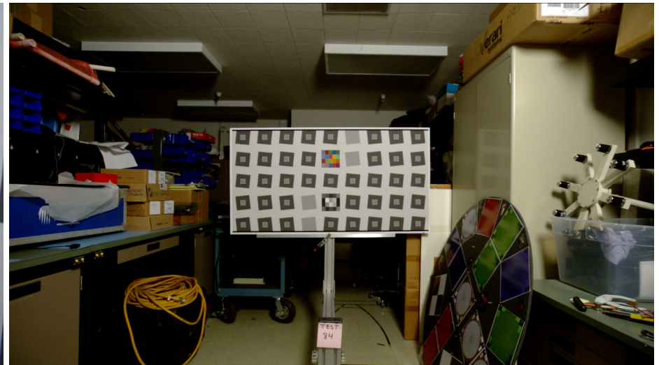
Ikegami HDL-50/HS, Zeiss 5mm Lens, 170 lux, 80 IRE, Target 112 inches (2.5m from dome equiv.), F 2.5, focus distance 35.5 inches File: Test_84.tiff
