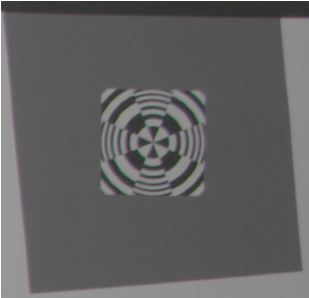
Sony F-55, Zeiss 12mm T2 Ultra Prime Lens, 840 lux, EI 1250, Target 34 inches, 4K P60 File: Test_111_4K.tiff
