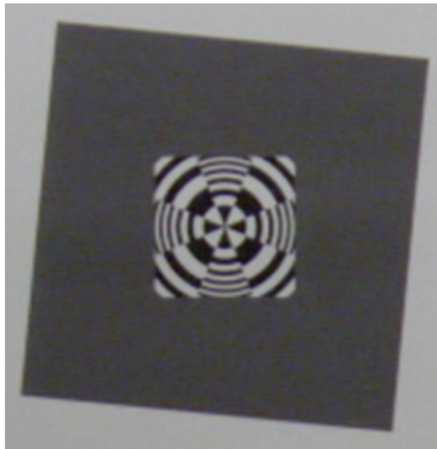
Ikegami HDL50/HS, 5mm Lens, 140 lux, 80 IRE, Target 39 inches File: Test_77.tiff
