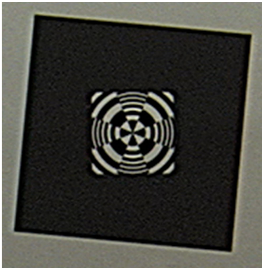
Ikegami HDL45, 5mm Lens, 110 lux, 80 IRE, Target 39.5 inches File: Test_100.tiff
