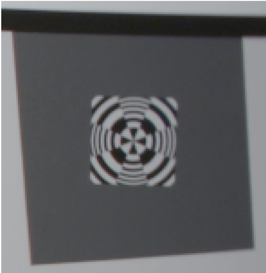
Sony F-5, Zeiss 12mm Lens, 400 lux, ISO 800, Target 34 inches, 1920x 1080 P60 (no color correction) File: Test_54_1920_4444.tiff
