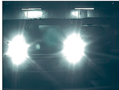
Vertical smear is reduced by the use of HAD sensor
