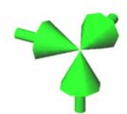
Node of solid or truss element: All three displacements are zero.
