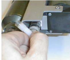
Rotate C Duct clockwise
