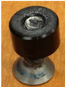
(shown with plunger switch removed) Grab connector end cap and rotate counter-clockwise
