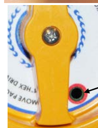
If removing battery pack from housing: Unthread post using 9/64 inch hex drive
