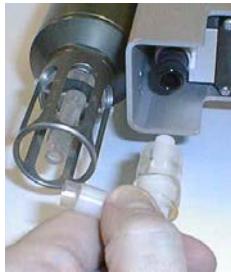
Pull C Duct straight out from conductivity cell
