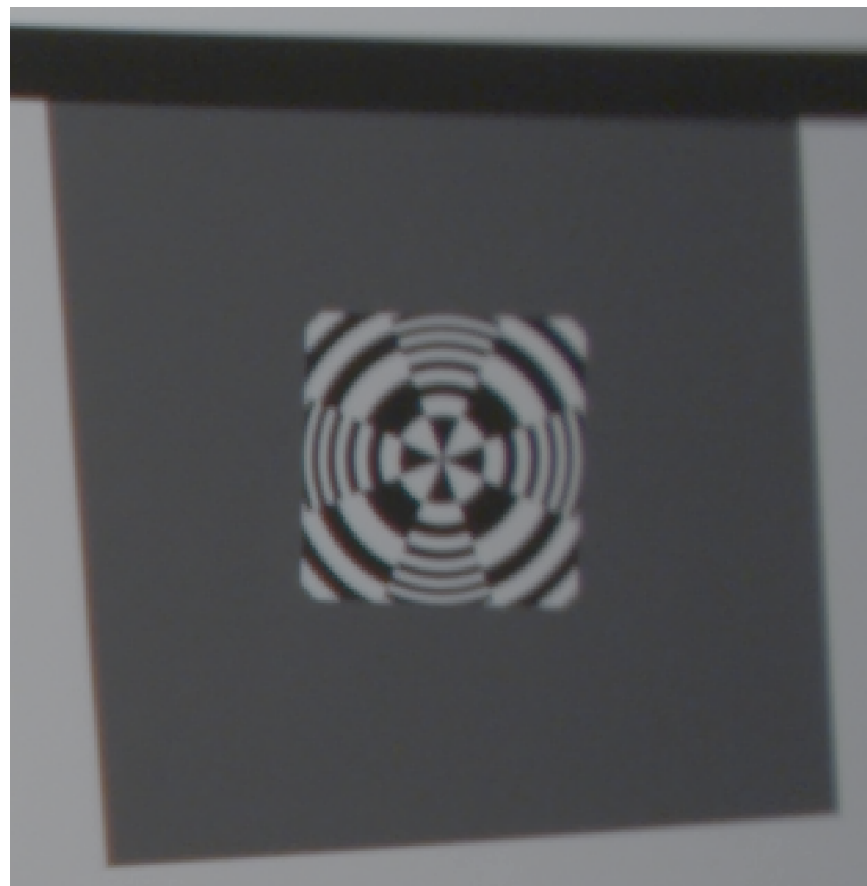
Sony F-5, Zeiss 12mm Lens, 800 lux, IE 2000, Target 34 inches, 4K P60 (no color correction)
