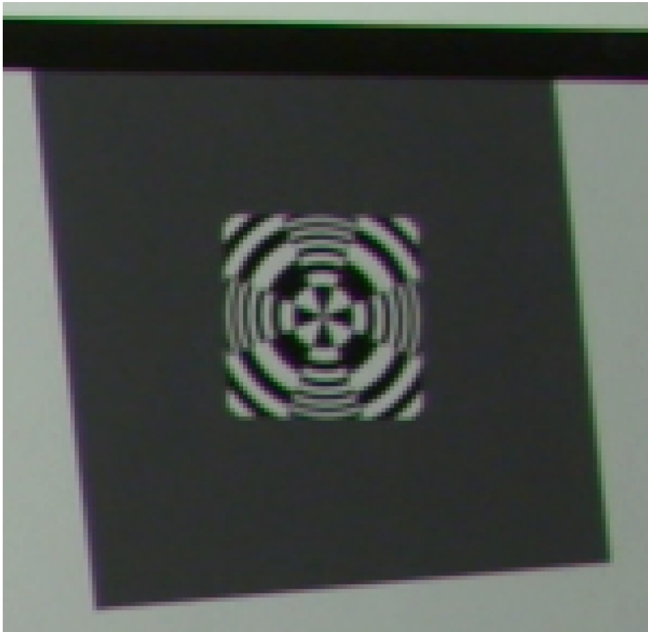
Sony F-5, Sony 11mm Lens, 400 lux, ISO 800, Target 36 inches, 1920x 1080 P60 File: Test_13X.tiff
