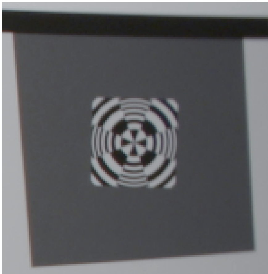
Sony F-5, Zeiss 12mm Lens, 400 lux, ISO 800, Target 34 inches, 1920x 1080 P60 (no color correction)
