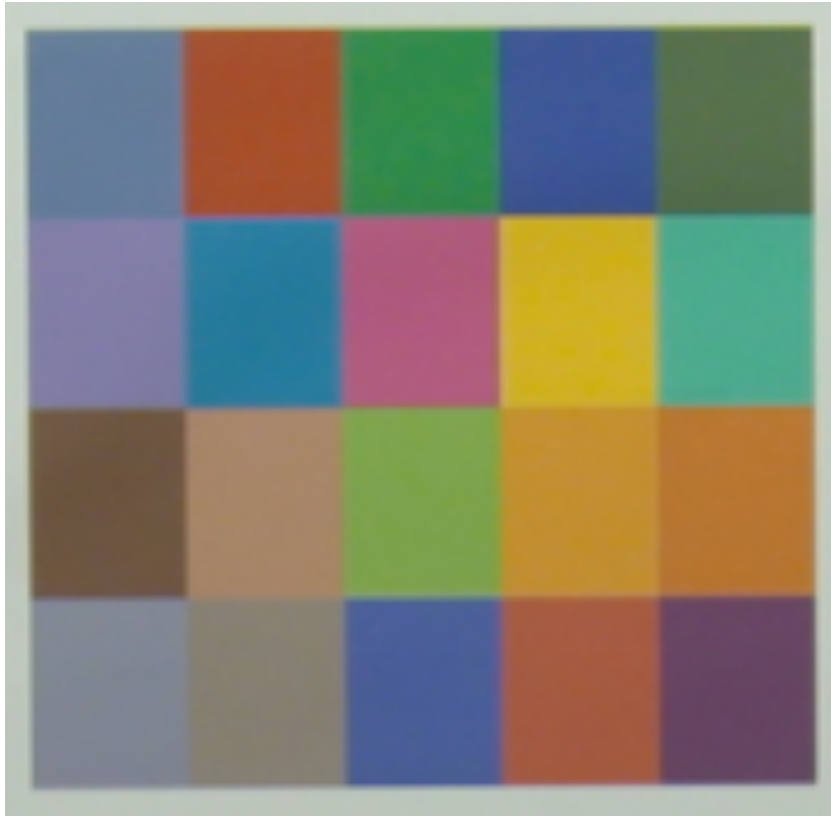
Sony F-5, Sony 11mm Lens, 400 lux, ISO 800, Target 36 inches, 1920x 1080 P60 (no color correction)
