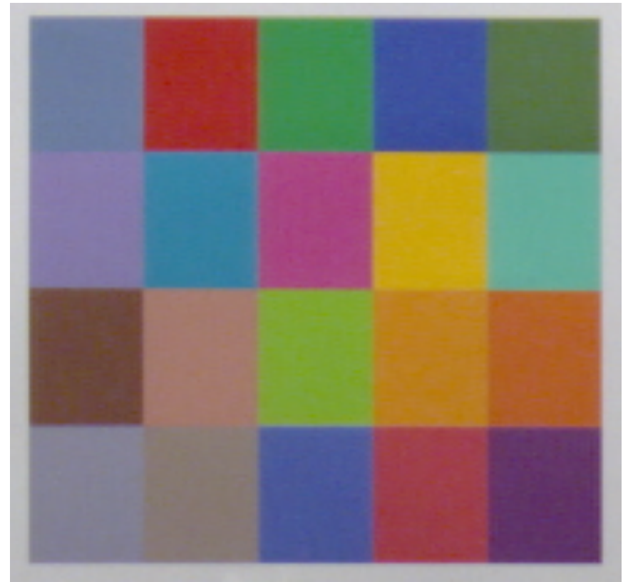
Ikegami HDL-50/HS, Zeiss 5mm Lens, 140 lux, 80 IRE, Target 38 inches (no color correction)
