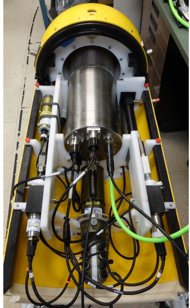
Fig. 10. The vehicle payload includes the camera housing, 2 Seabird CTDO sensors, 1 Seabird data logger, and 1 Wetlabs transmissometer.
