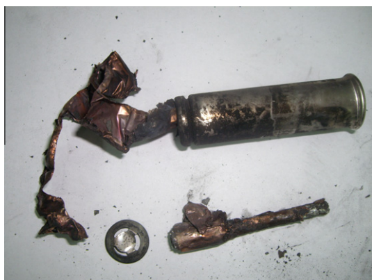
Fig. 1. The LiCoO 2 material battery was destroyed by VSP2 trials.
