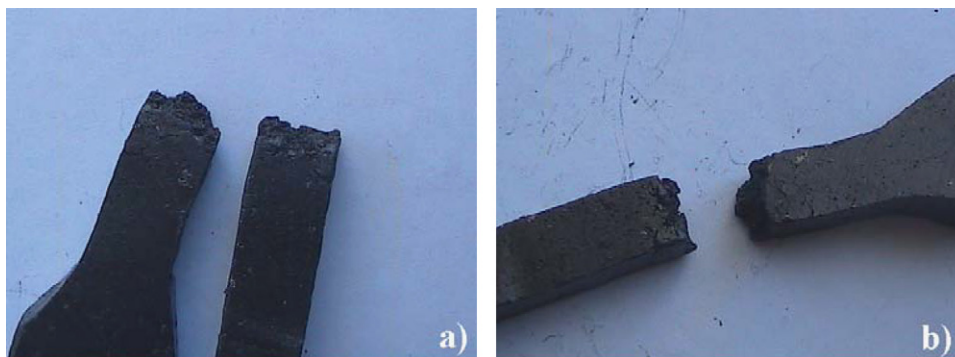
Fig. 7. fractured samples in the tensile test: (a) Sample impregnated for 12 h and tested at room temperature (Brittle fracture); and (b) sample impregnated for 12 h and tested at 45 °C (Ductile fracture).
