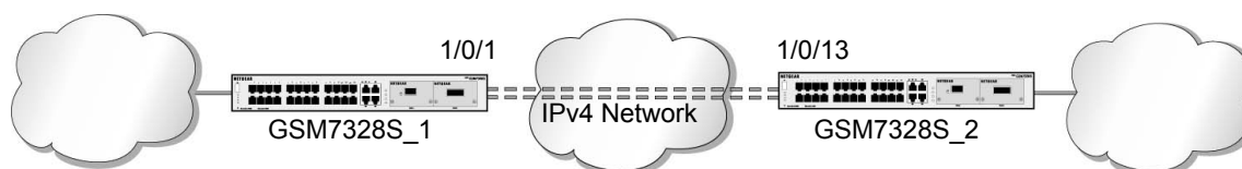
Figure 44. 6in4 tunnel between two switches
