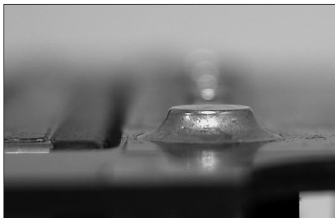
Figure 14-1 — Side profile of a Mini module solder joint
