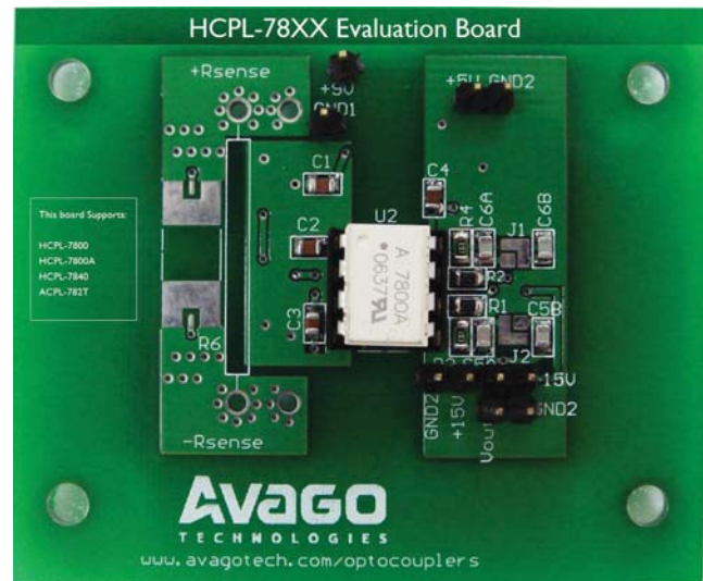
Figure 1. HCPL-7800A/7800/7840 & ACPL-782T Evaluation Board (Top View)
