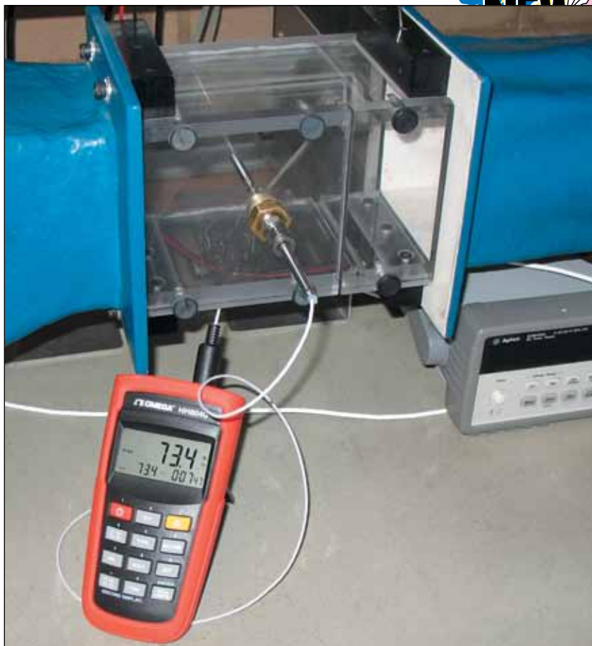
P-L-A-1/4-6-0-T-3 Class A Air Sensor with optional HH804U hand held meter shown smaller than actual size. For more information on HH804U visit omega.com/hh804u
