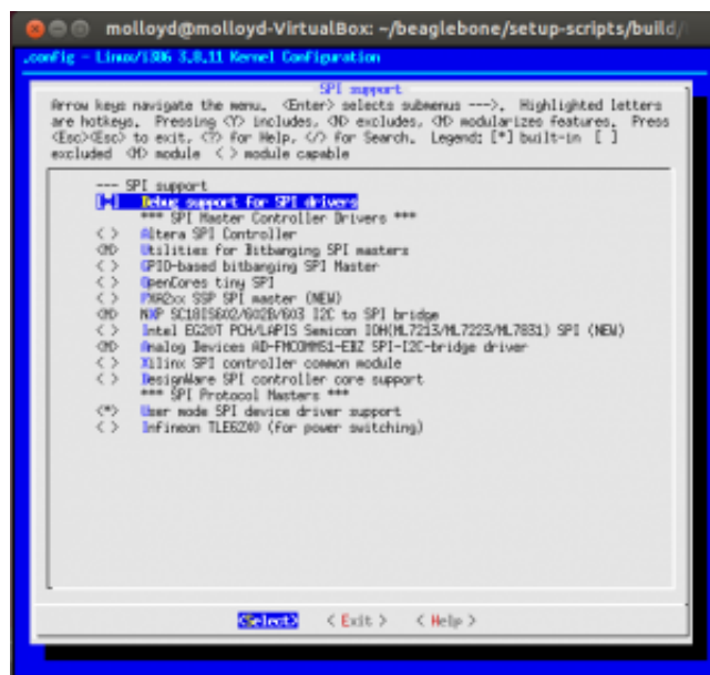
Figure 2: Enable “Debug support for SPI drivers” by pressing ‘Y’
