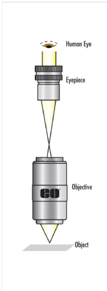
Figure 11: Simplified Finite Conjugate Microscope Design [ View Larger Image ]
