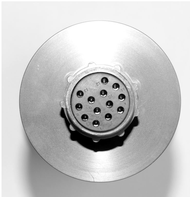
Submersible Microscope bulkhead with 13 pin connector
