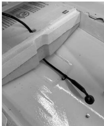
Figure 9.15. Installing the GPCTD Cable
