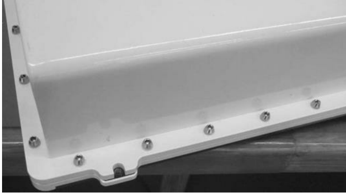
Figure 9.18. Installing the Payload dry box Lid Assembly Attachment Screws
