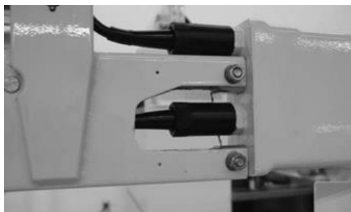
Figure 9.34. GPCTD Subconn Connector to Glider with Cable Clamp
