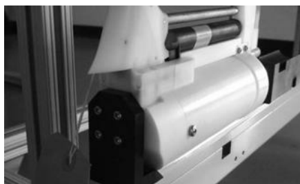
Figure 9.30. GPCTD Bracket and Attachment Screws
