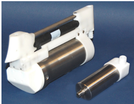
GPCTD with pump (shown with optional 1500 m titanium housing)
