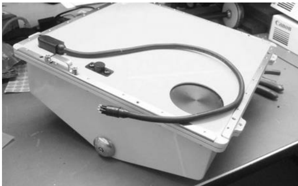
Figure 9.19. Connecting the Payload Cable to the C&C
