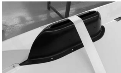
Figure 9.14. Attaching the GPCTD Housing Screws
