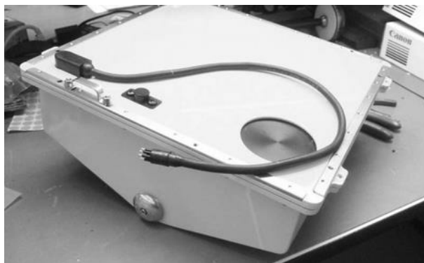
Figure 9.9. Payload Drybox and C&C Connection Cable
