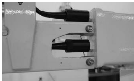
Figure 9.25. GPCTD SubConn Connector to Glider with Cable Clamp
