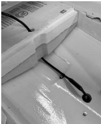
Figure 9.12. Removing the GPCTD Cable
