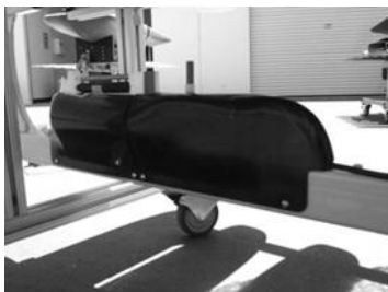
Figure 9.33. GPCTD Front and Back Fairings
