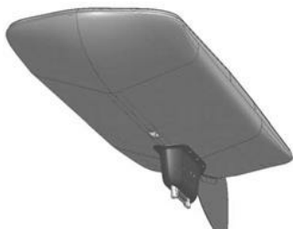
Figure 1.2. GPCTD Attached To Glider
