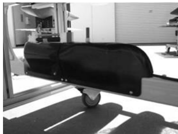
Figure 9.26. GPCTD Front and Back Fairings
