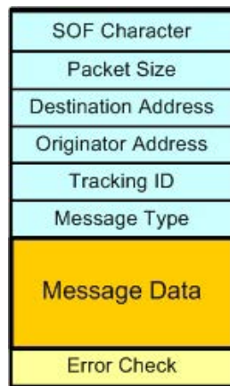
Figure 8.1. Payload Data Packet Format
