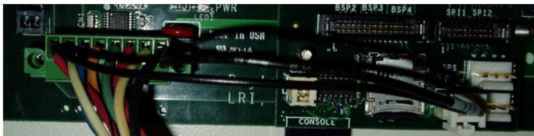
Figure 10.8. GPS/PPS Connections to a PIB
