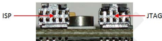
Figure 10.31. ISP Pin Number Orientation
