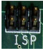
Figure 10.16. Atmel ISP - J5 Pin Number Orientation
