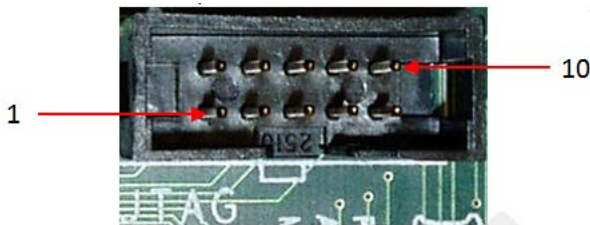
Figure 10.19. Atmel JTAG - J4 Pin Number Orientation
