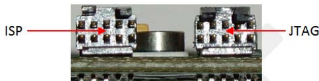
Figure 10.36. JTAG Pin Number Orientation
