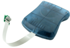
Figure 10.38. Atmel ATJTAGICE2 without the Programming Adapter
