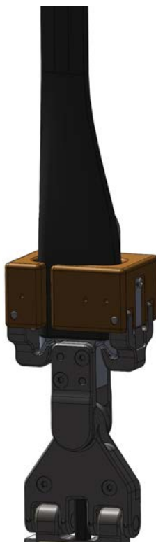
Figure 2.12. Glider Recovery Mechanism Locked Onto Recovery Hooks
