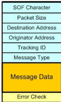
Figure 8.1. Payload Data Packet Format
