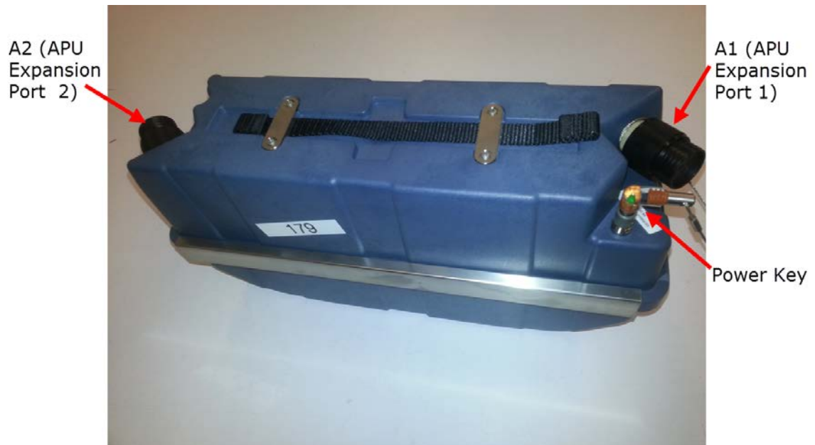
Figure 3.17. Auxiliary Power Unit (APU) Electrical Connections
