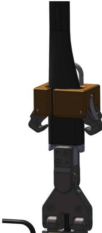
Figure 2.11. Glider Recovery Mechanism
