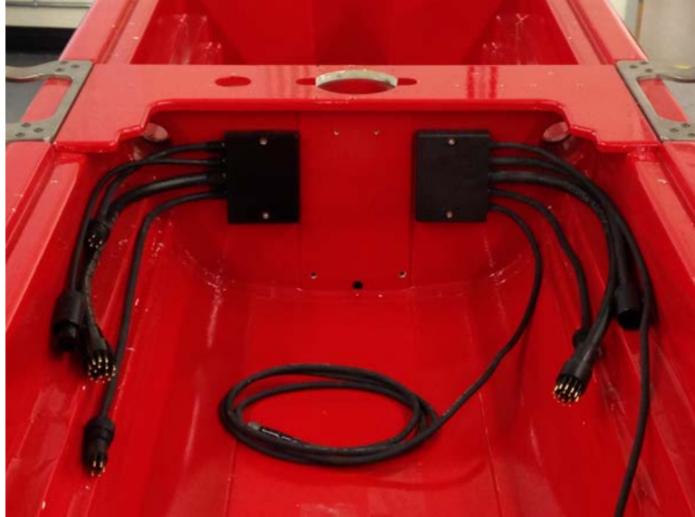
Figure 3.10. Octopus Cable Assemblies Mounted to Bulkhead
