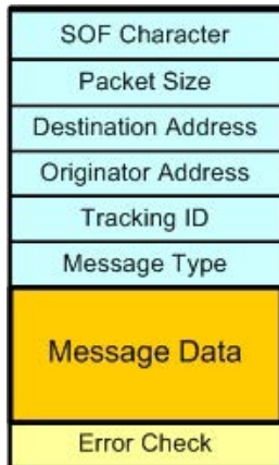
Figure 8.1. Payload Data Packet Format
