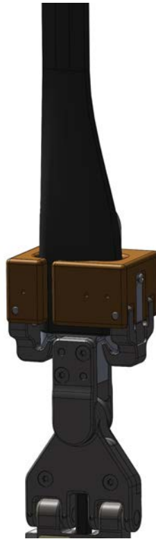
Figure 2.12. Glider Recovery Mechanism Locked Onto Recovery Hooks
