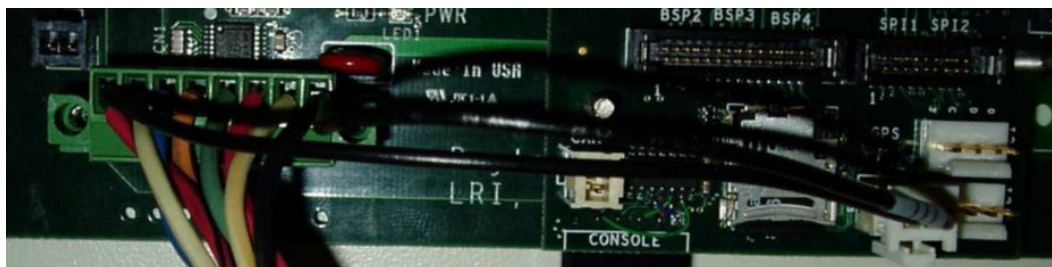
Figure 10.19. GPS/PPS Connections to a PIB
