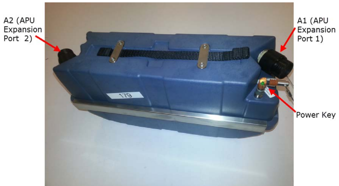
Figure 3.17. Auxiliary Power Unit (APU) Electrical Connections
