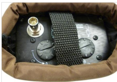
Figure 9-4: Battery Covers on Bottom of Receiver
