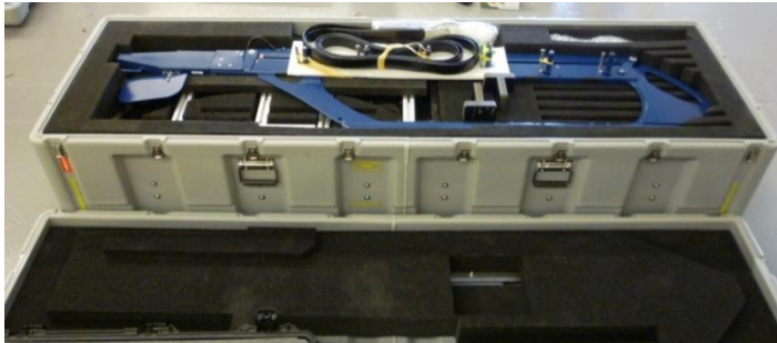
Figure 3-1: Glider Container Contents
