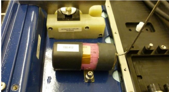
Figure 9-1: Emergency Radio Beacon
