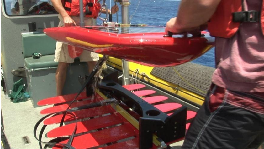
Figure 8-6: Float Being Set Down on Saddle
