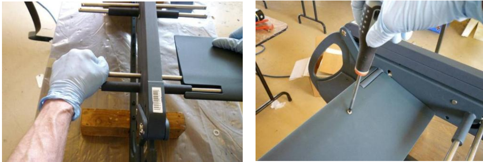
Figure 3-4: Installing and Securing Wing
