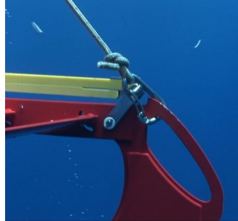
Figure 8-2: Recovery Line Attached To Glider Nose
