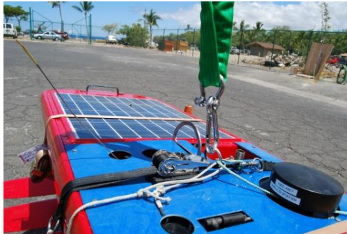
Figure 6-4: Lifting Using Release Strap
