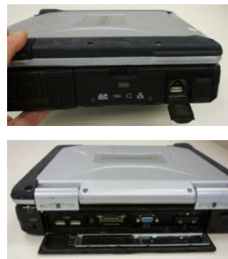
Figure 2-4: Toughbook, Showing Side and Back USB Ports
