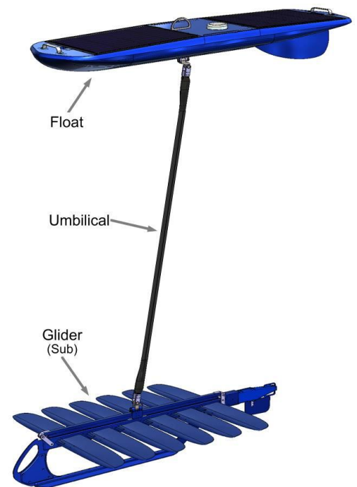
Figure 1-3: Wave Glider Main Components
