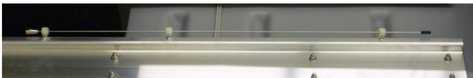
Figure 3-20: AIS Antenna Shipped in Float Case Lid
