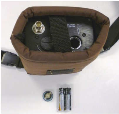
Figure 9-7: Battery Compartment Cover Removed
