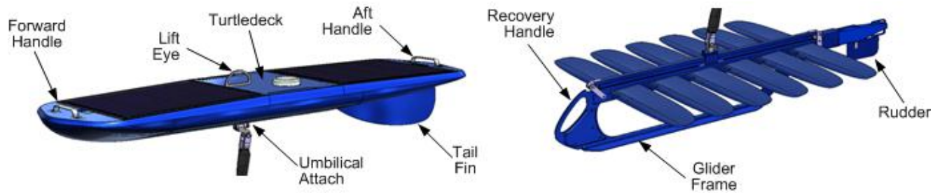
Figure 1-4: Float and Glider Primary External Parts
