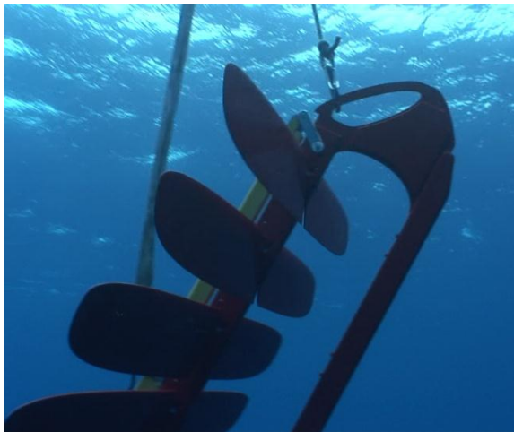
Figure 8-3: Glider Hoisted Vertically to Disable Forward Motion
