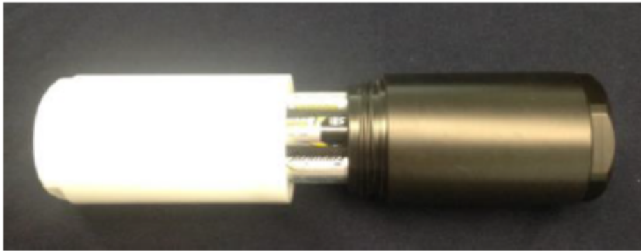
Figure 5.1. Unscrew Resilient Tracker Housing
