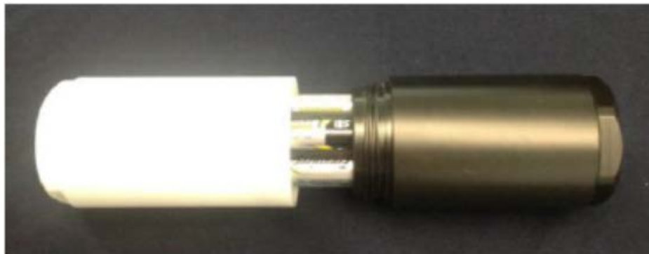
Figure 5.1. Unscrew Resilient Tracker Housing
