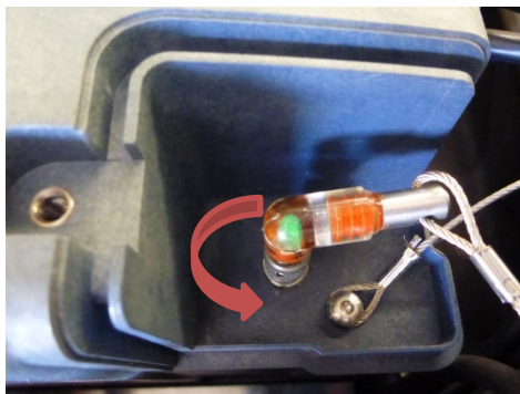
Figure 3: SV3 Power Key (Turn retaining ring counter clockwise)
