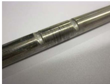
Figure 16: Damaged/Worn Shaft (Wear >0.5mm)
