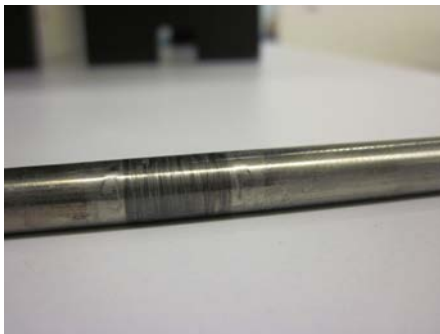
Figure 15: Acceptable Wear on Shaft
