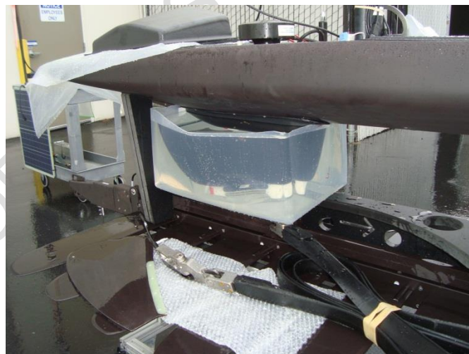
Figure 46: Move Sub-CTD to Fresh Water Tank
