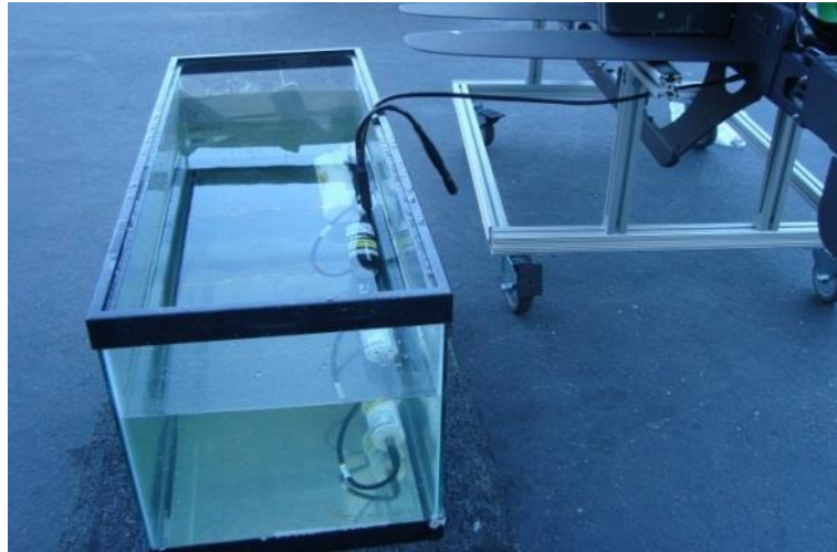
Figure 45: Move Sub-CTD to Fresh Water Tank
