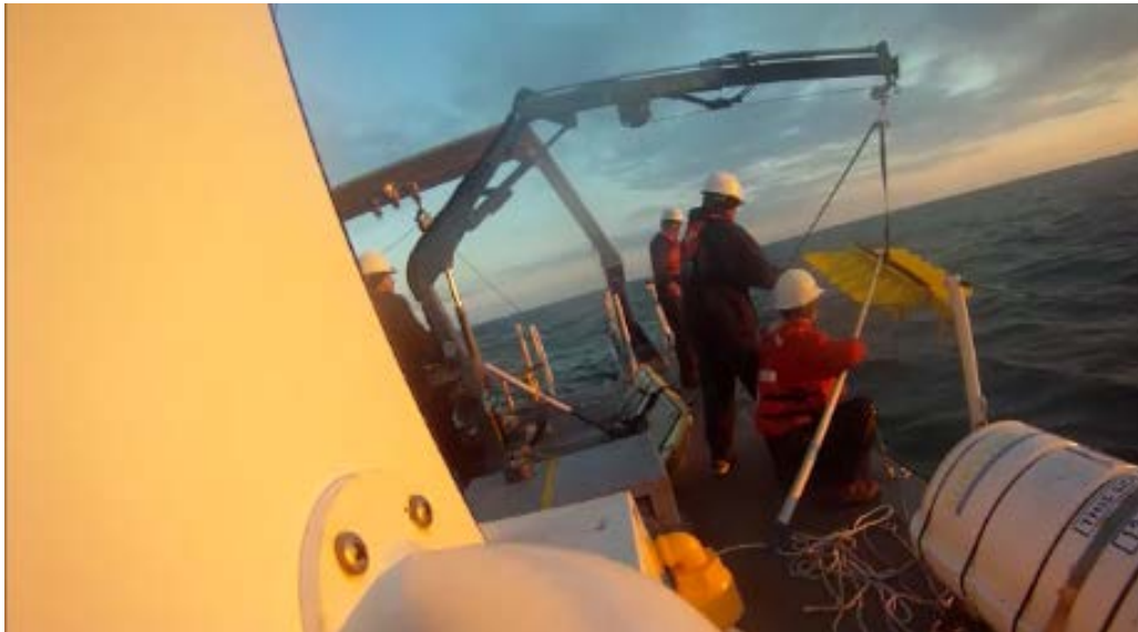
Figure 9.36. Connect Hoisting Line to the Sub Recovery Device and Hoist the Sub
