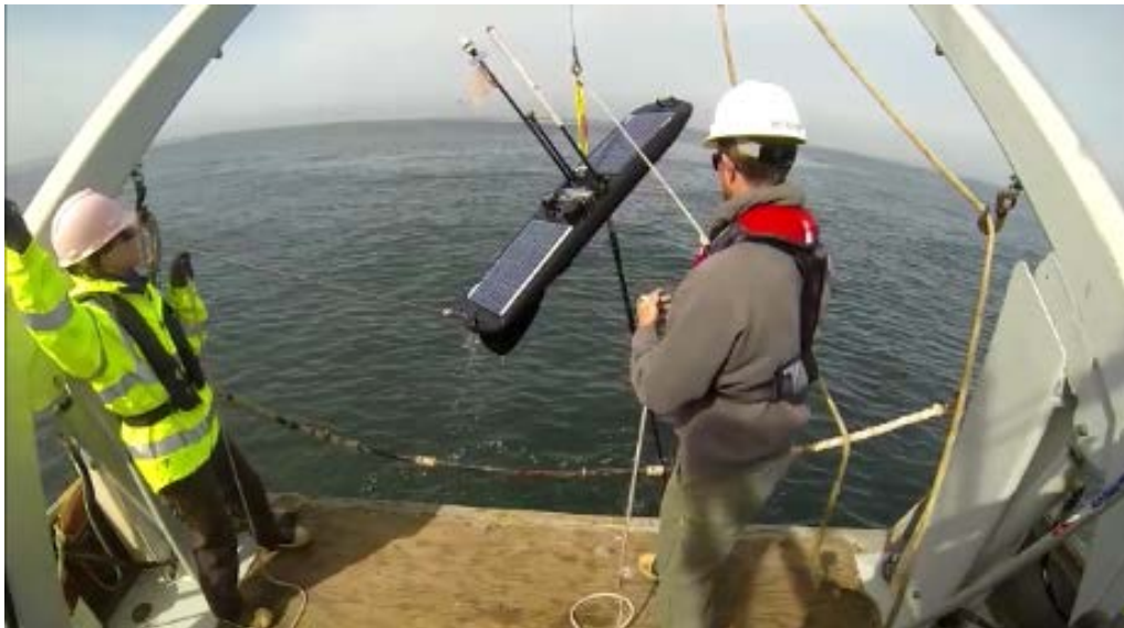
Figure 9.23. Hoist Operator Lifts the Float out of the Water
