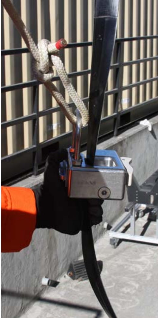
Figure 9.25. Attaching Sub Recovery Device to Umbilical 2
