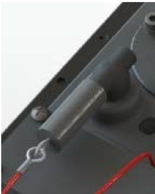
Figure 7.1. Shorting Pin (Power Key) Installed
