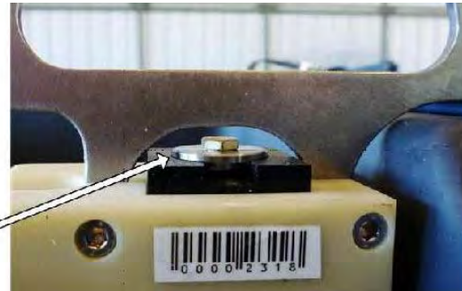
The metal disk must be raised above the black plastic base.
