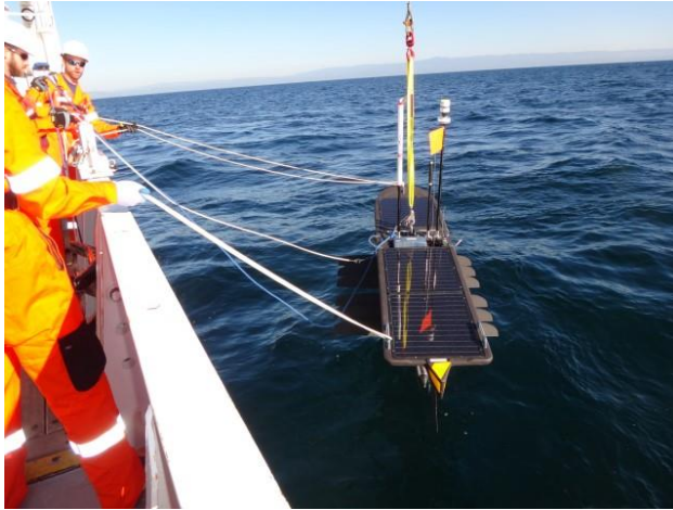
Figure 8.8. Bow of the Wave Glider is Oriented Away from Vessel
