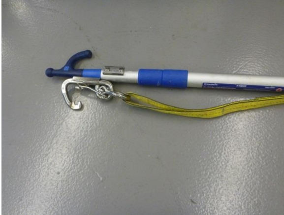
Figure 6.9. Boat Pole with Carabiner Clip and Lift Strap
