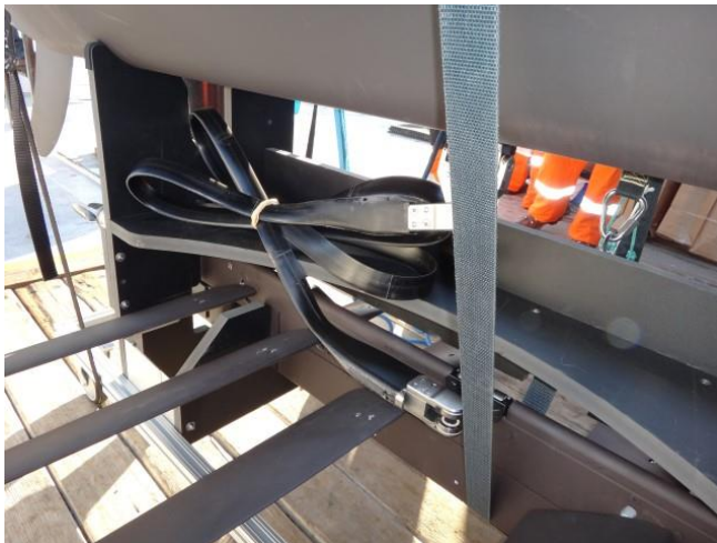
Figure 8.5. Umbilical Stowed for Launch
