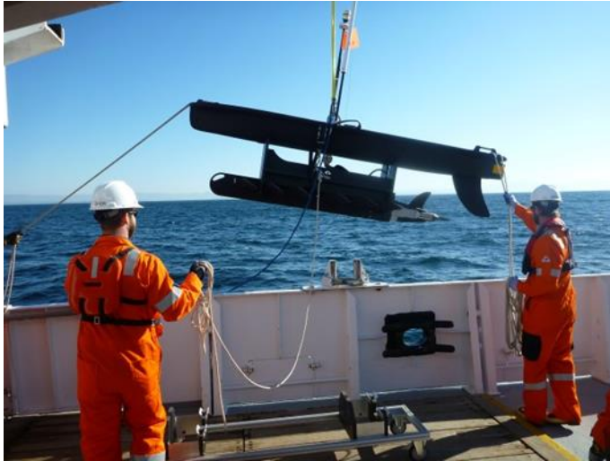
Figure 2.2. Wave Glider SV3 Bundled during Launch
