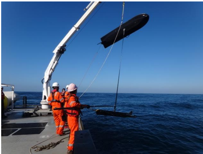
Figure 9.8. Continue Hoisting Until the Sub Clears the Rail
