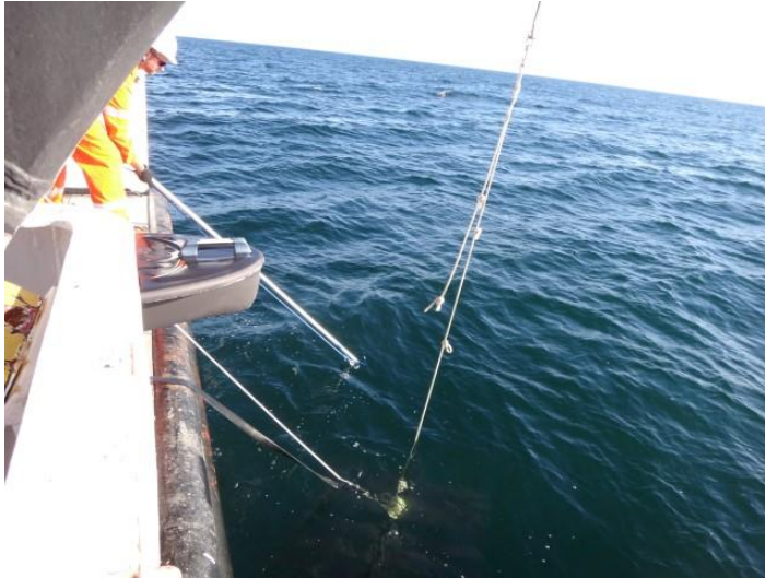
Figure 9.20 Connect a Tag Line to the Bow of the Sub
