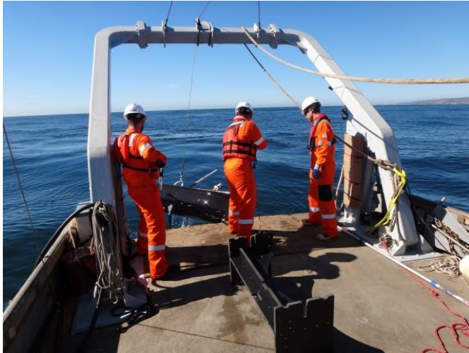
Figure 9.12. Hoist the Float out of the Water to Access Umbilical
