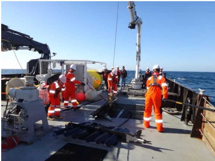
Figure 9.10. Lower Float to Deck
