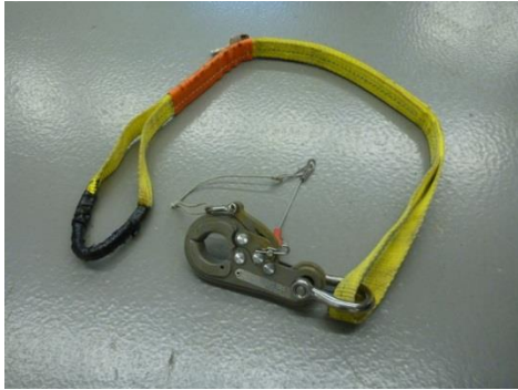
Figure 6.2. SeaCatch with Lift Strap
