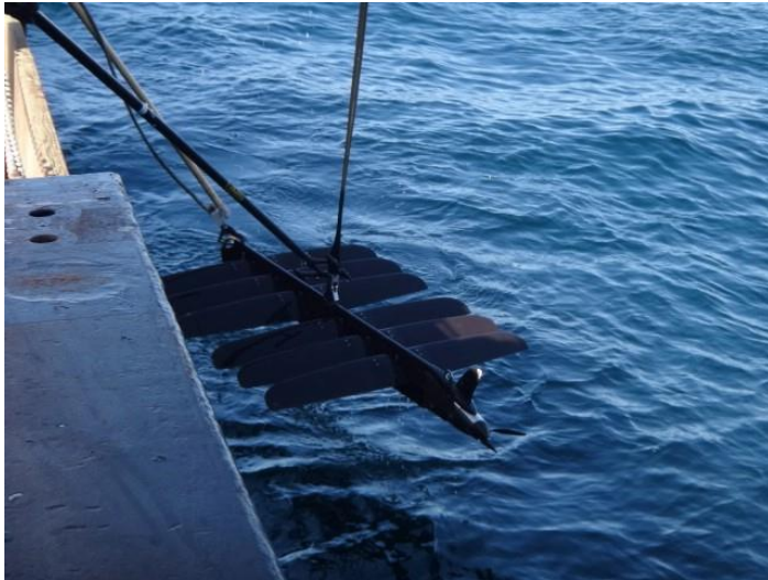
Figure 9.8. Continue Hoisting Until the Sub Clears the Rail
