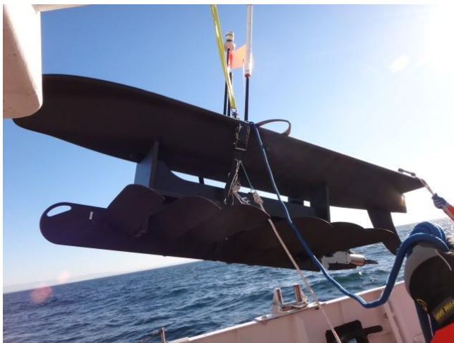
Figure 8.7 Wave Glider Hoisted for Launch
