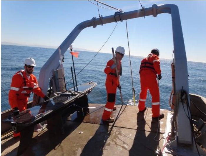
Figure 9.14. Attach Tag Line to Bow of Sub
