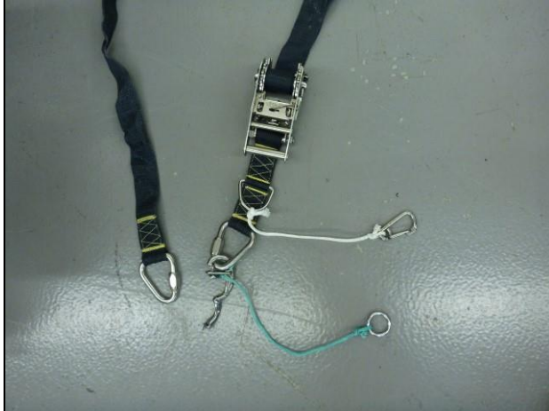
Figure 8.3. Bundling Strap with Quick Release Shackle Latched
