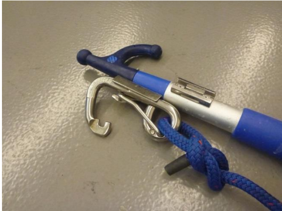
Figure 6.8. Boat Pole with Carabiner Clip and Tag Line
