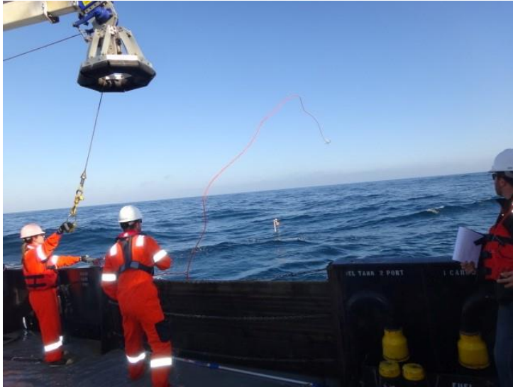
Figure 9.2. Grappling the Recovery Buoy Line
