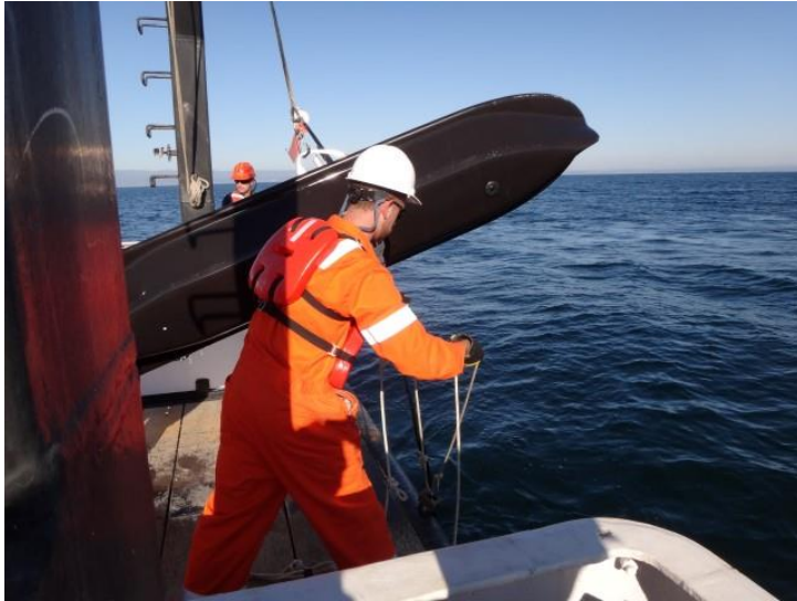
Figure 9.18 Hoist the Float as High as Possible; Tie off the Sub Recovery Device Tag Line
