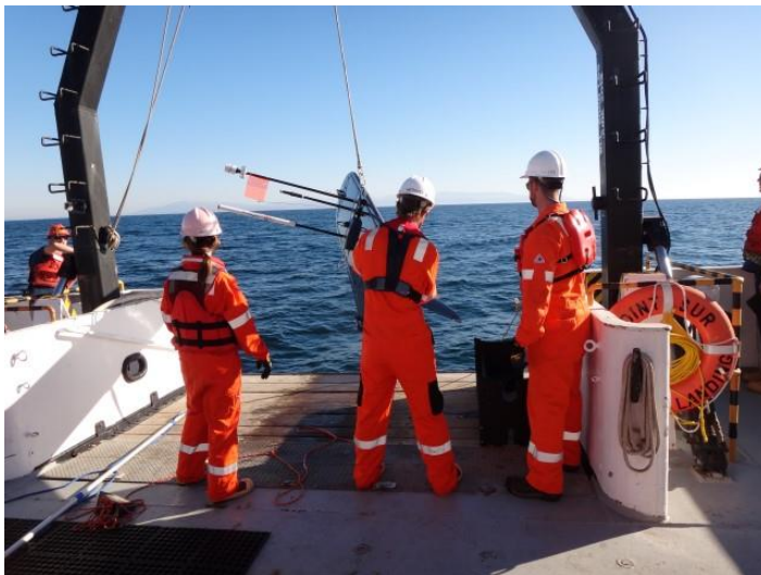
Figure 9.18 Hoist the Float as High as Possible; Tie off the Sub Recovery Device Tag Line
