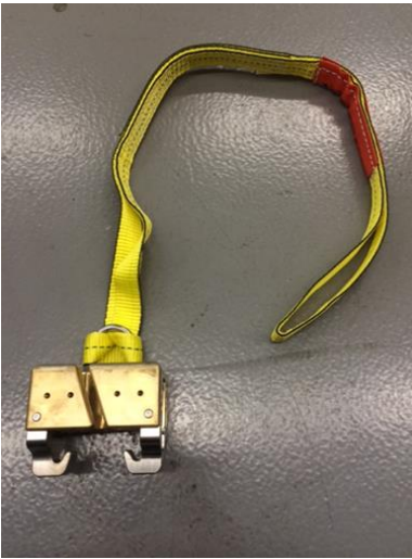
Figure 4.1. Sub Recovery Device with Lift Strap
