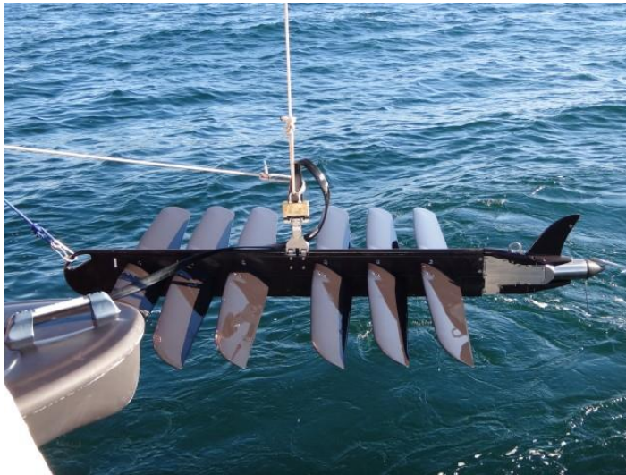
Figure 9.20 Connect a Tag Line to the Bow of the Sub
