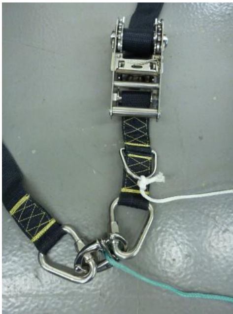
Figure 8.3. Bundling Strap with Quick Release Shackle Latched
