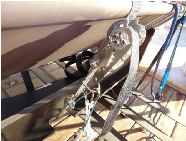
Figure 8.5. Umbilical Stowed for Launch
