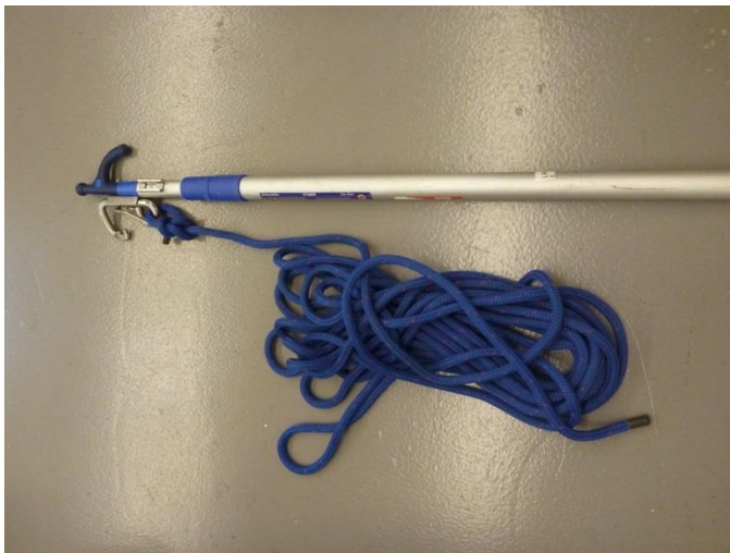
Figure 6.8. Boat Pole with Carabiner Clip and Tag Line
