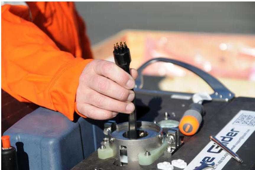
Figure 9.6. Pull the Umbilical Whip Through the Motion Isolator
