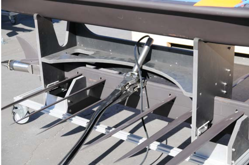
Figure 9.5. Position the Umbilical Motion Isolator Shaft for Insertion
