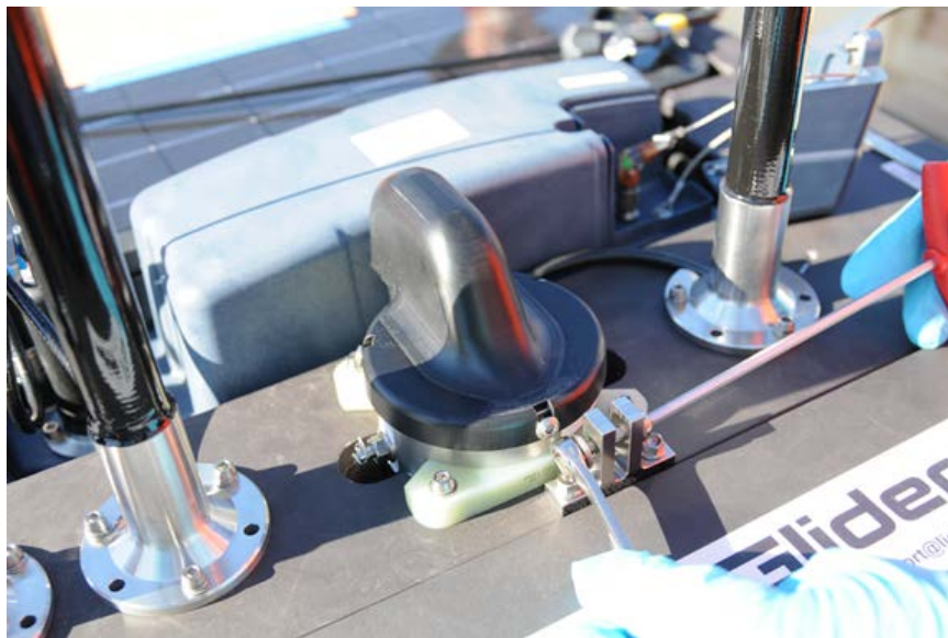
Figure 11.1. Remove Screws from the Lifting Ring Mounts
