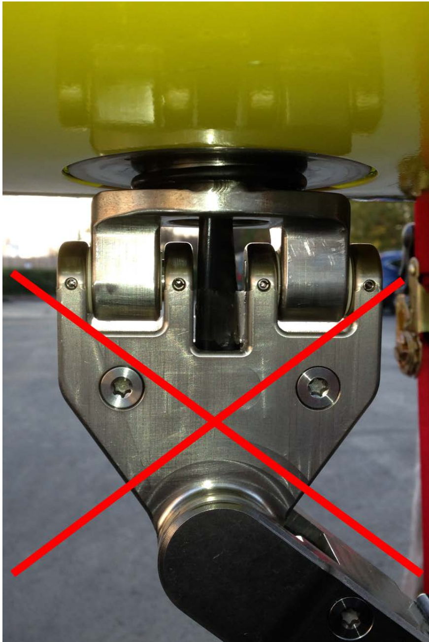
Figure 9.12. Ribbon Cable Rotated More Than 1/4 Turn at Top of Motion Isolator Shaft
