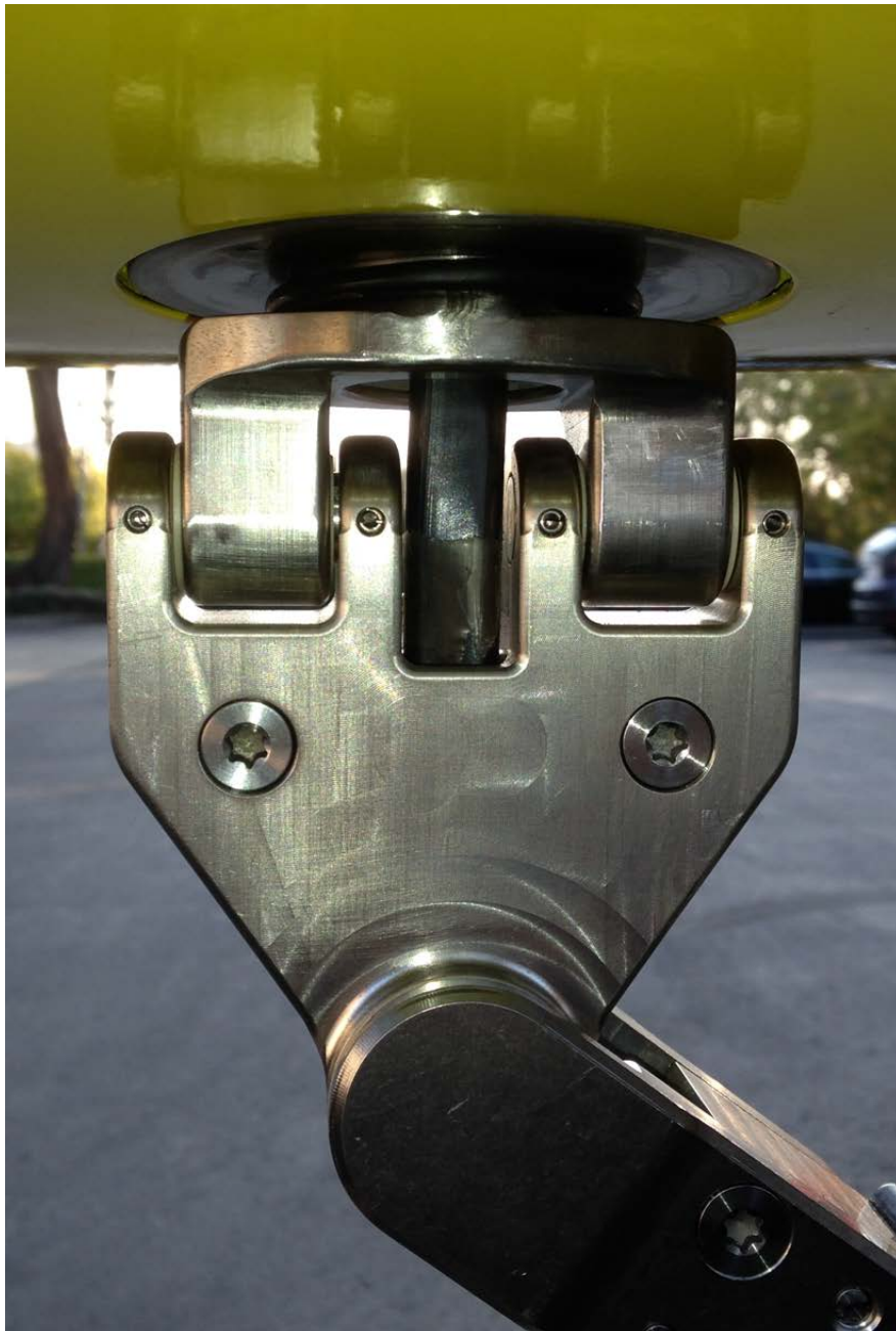
Figure 9.11. Ribbon Cable Rotated 1/4 Turn at Top of the Motion Isolator Shaft
