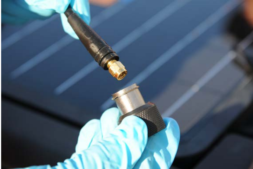
Figure 11.9. Slide Cell Antenna Connector Through the Retainer
