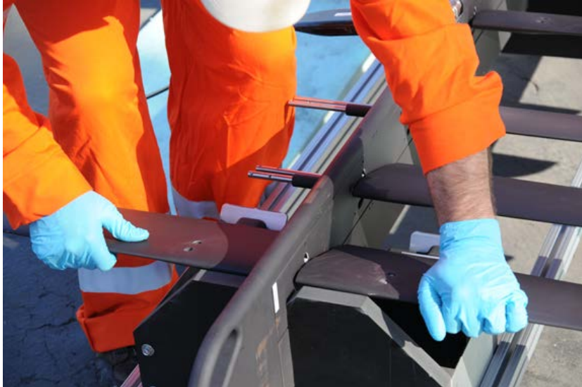
Figure 6.9. Slide the Second Wing in the Wing Pair onto the Pivot and Spring Shafts
