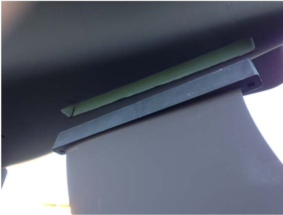
Figure 8.16. Insert Skeg Into Slot Under the Aft End of the Float
