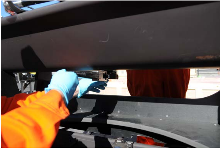
Figure 9.9. Hold the Umbilical Motion Isolator Shaft in Position
