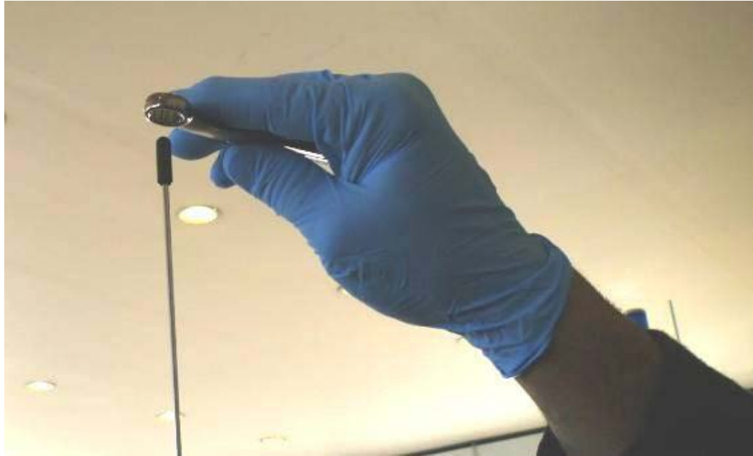
Figure 11.14. Tighten AIS Antenna
