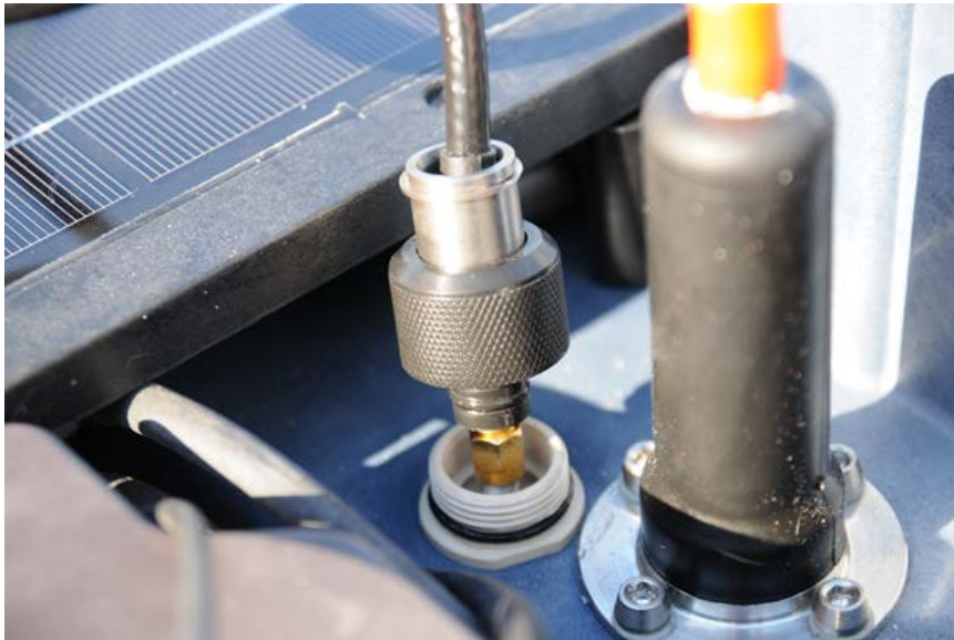
5. Figure 11.12. Hand-Tighten the Black Retainer Ring
