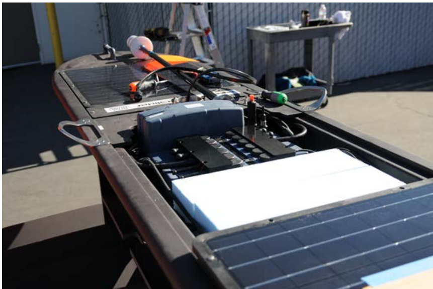
Figure 9.16. Remove the Center Solar Panel
