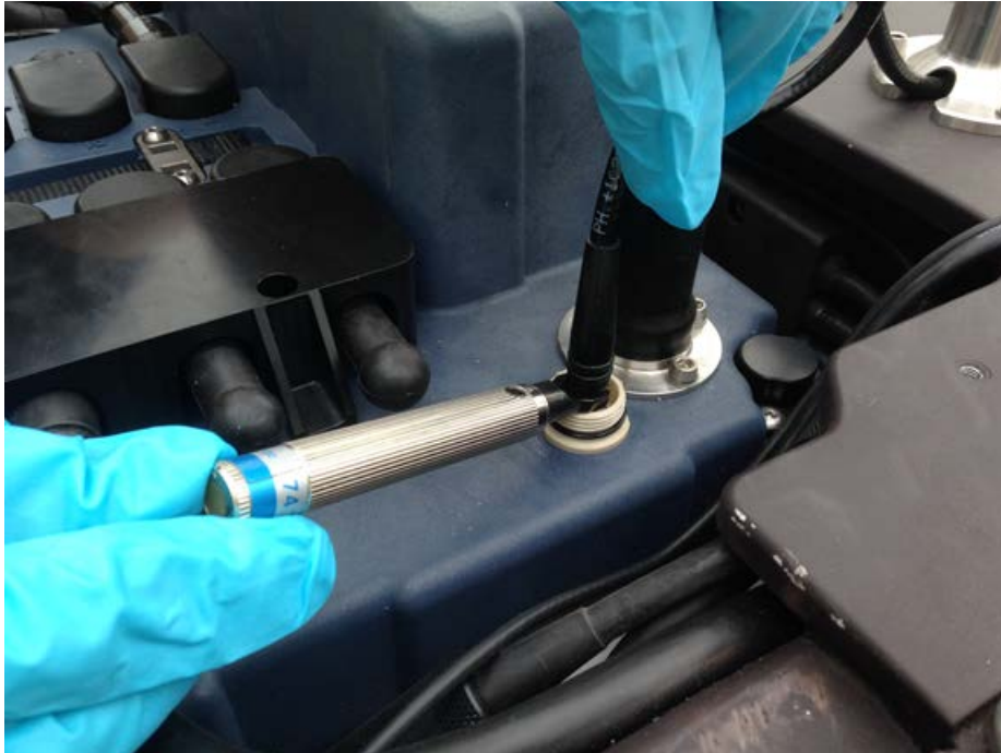
Figure 11.10. Connect the Cell Antenna Cable
