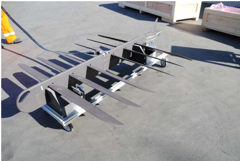
Figure 6.12. Sub Frame on Launch Stand with all Wings Installed
