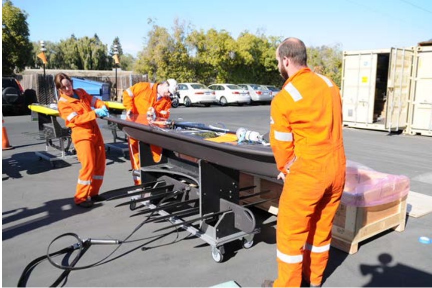
Figure 8.9. Align the Float on the Launch Saddle
