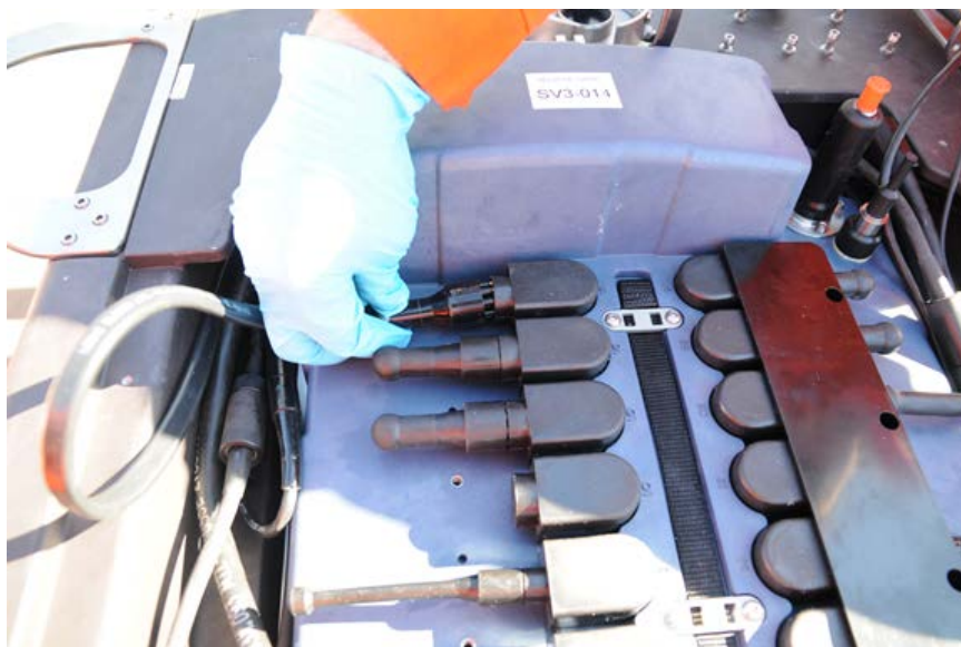
Figure 9.22. Connect the Umbilical Whip to the CCU
