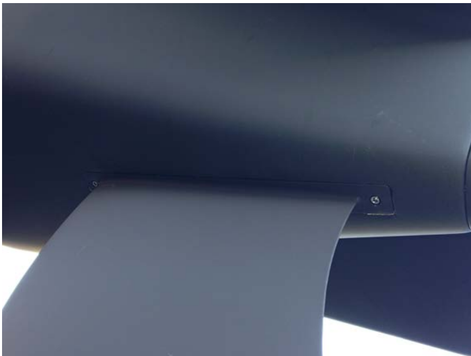
Figure 8.17. Secure Skeg with Two Screws
