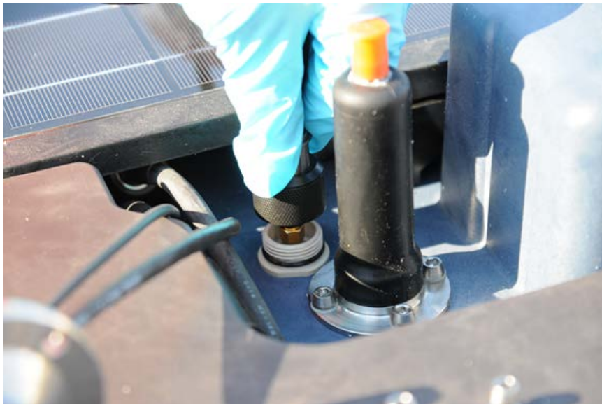
5. Figure 11.12. Hand-Tighten the Black Retainer Ring
