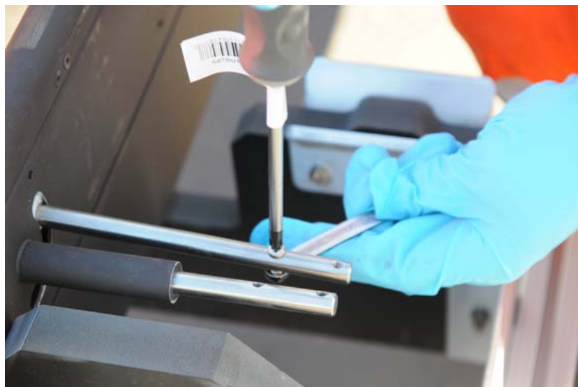
Figure 6.5. Removing Screws from Spring Shafts
