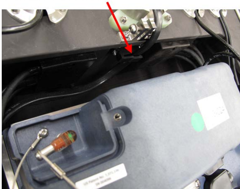
Figure 9.22. Connect the Umbilical Whip to the CCU
