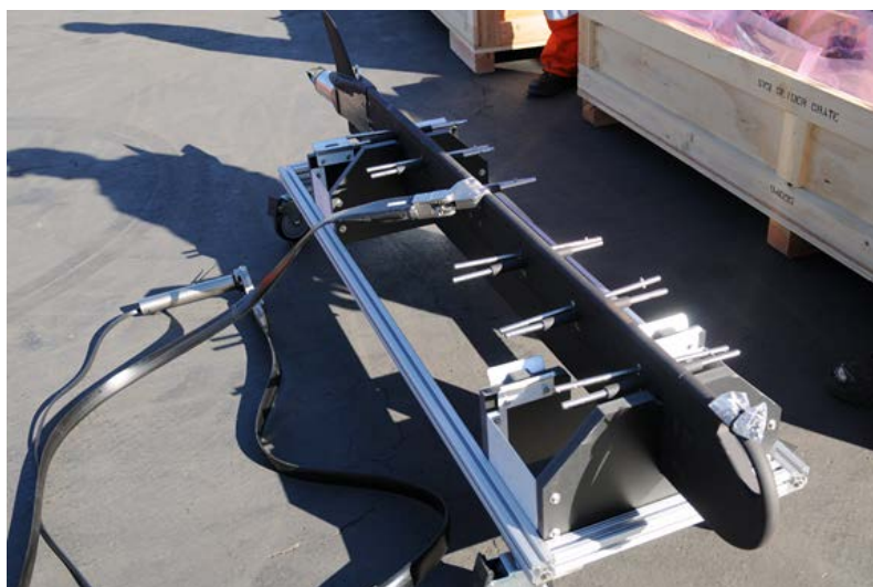
Figure 5.5. Sub Frame in Launch Stand with Umbilical Resting to Starboard Side
