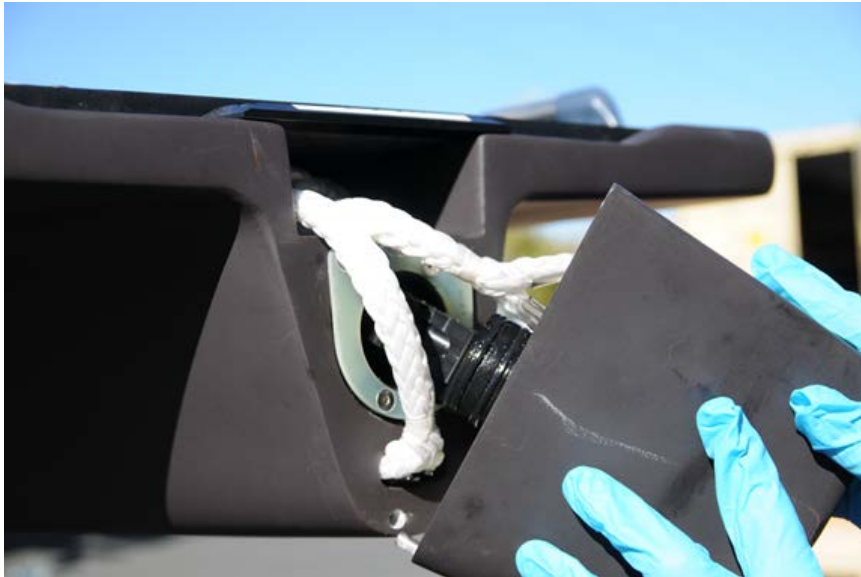
Figure 8.12. Insert Recovery Buoy Piston into Receptacle
