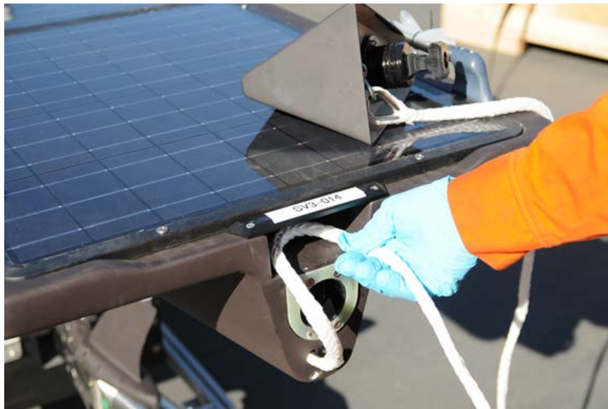
Figure 8.11. Feed the Recovery Buoy Tether into the Tether Cavity
