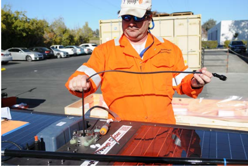
Figure 9.7. Remove Slack from the Umbilical Whip
