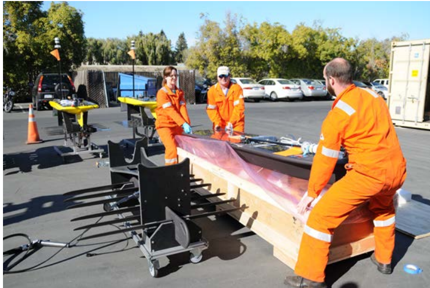
Figure 8.8. Place the Float on the Launch Saddle
