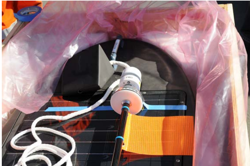
Figure 8.6. Recovery Buoy and Weather Station Mast Secured for Float Lifting
