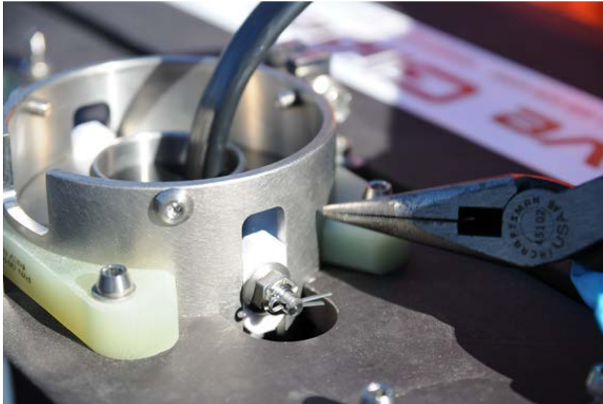
Figure 9.15. Install the Cotter Pin
