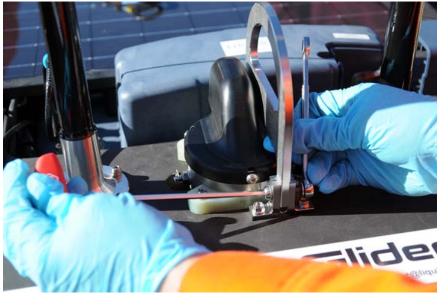
Figure 11.2. Install Screws in Lifting Ring Mount
