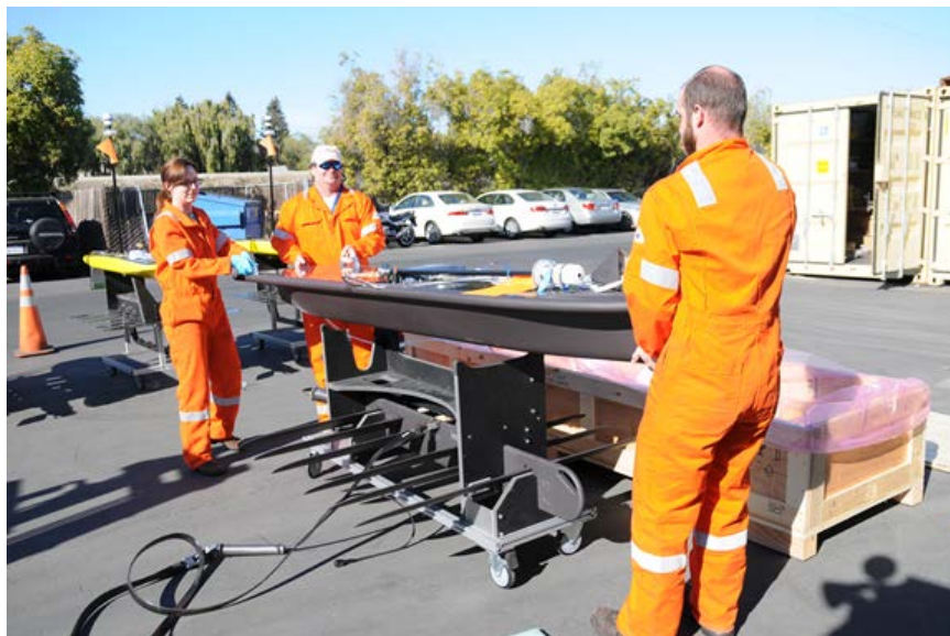
Figure 8.8. Place the Float on the Launch Saddle
