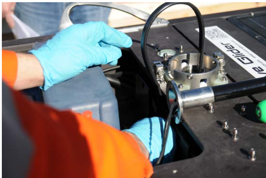
Figure 9.20. Slide the CCU Forward
