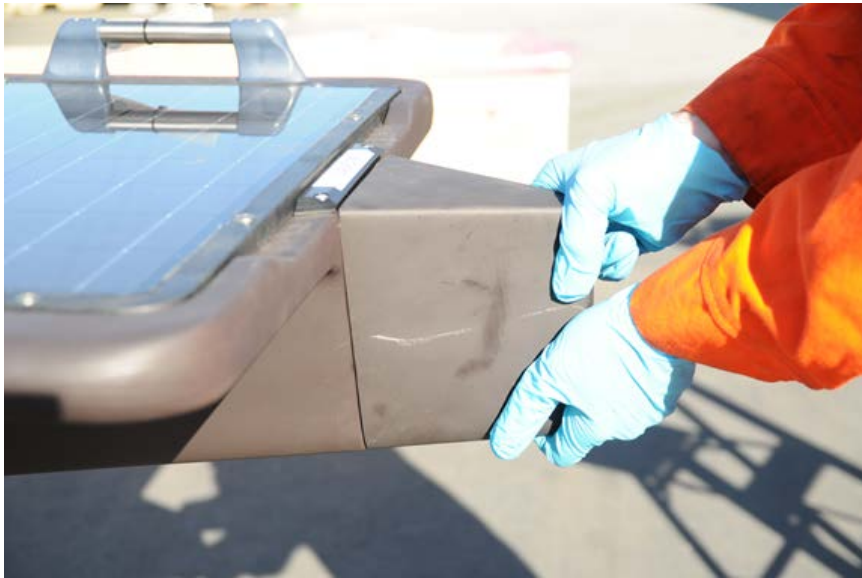
Figure 8.14. Properly Installed Recovery Buoy
