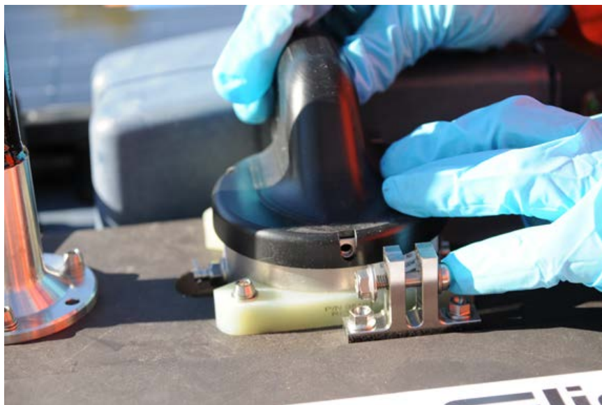
Figure 9.28. Install Umbilical Whip Shroud
