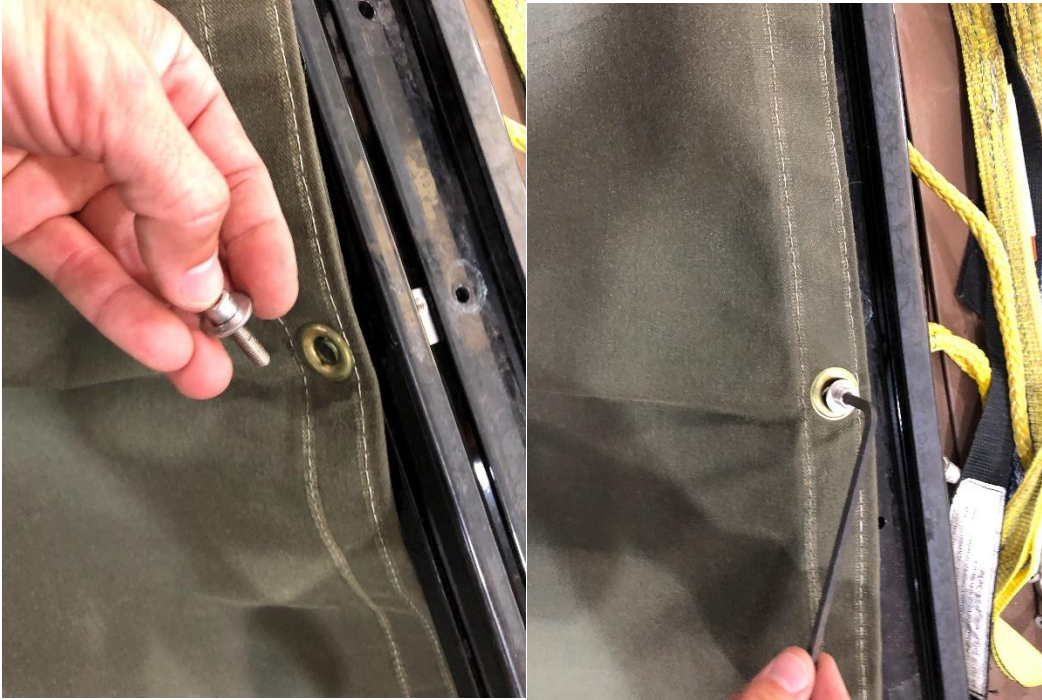
Figure 88. Secure each pair of eyes in the tarpaulin with a M6 screw and washer.
