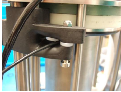
Figure 63. Secure the shoulder screw, nylock, and nylon spacer. Slip the Thin Line out of the gap. Tighten the nut until there is still about 0.5 mm side to side movement of the shoulder screw.
