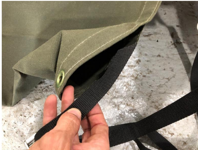
Figure 91. Route the strap through the slot in the tarpaulin.
