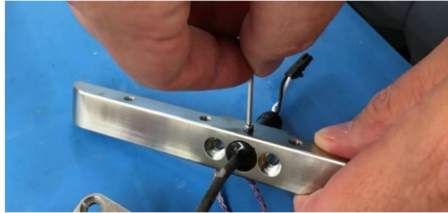
Figure 70. Remove and store the two set screws securing the penetrator in place.
