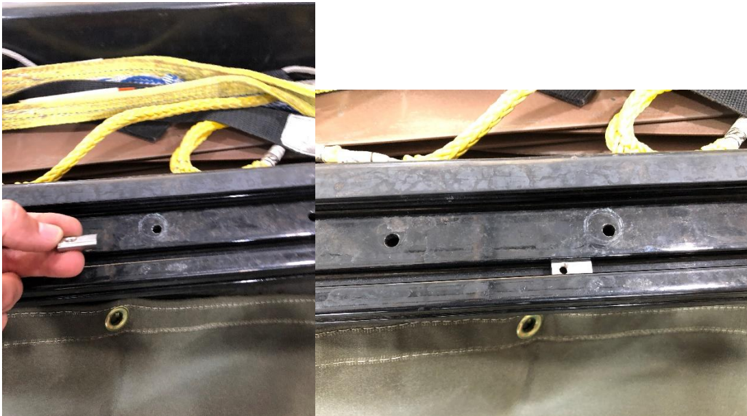
Figure 87. T-Nuts placed in the crossmember channel with flat side up.
