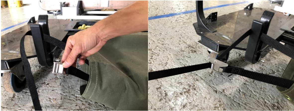
Figure 92. Strap routed through the front sub cradle slot and through the strap cam.
