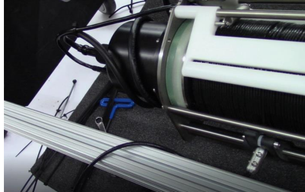
Figure 41. Excess cable wrapped around the Winch body.
