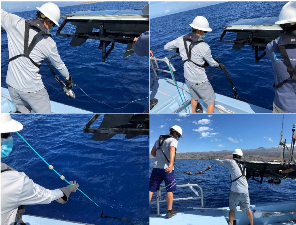
Figure 23. The Sinker should be placed over the freeboard and kept from free-falling into position (A). Lower the Sinker gently using the Tow Cable or drogue (whichever is directly attached to the Sinker) until it is fully supported by the Thin Line (B, C, D). Verify that the Sinker and Thin Line are suspended unencumbered from the Winch.
