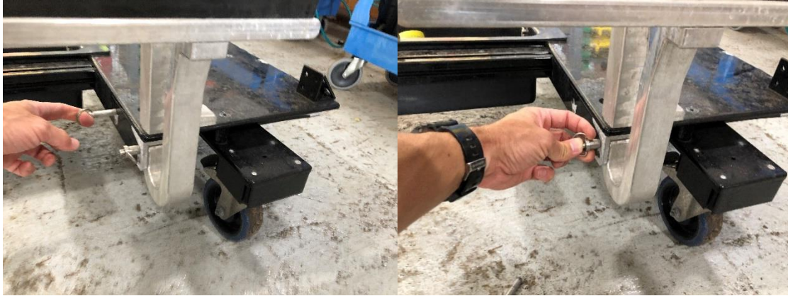
Figure 82. Rapid cart with L-Drop adapter Kit installed.
