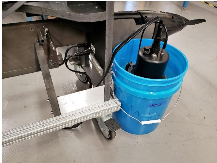
Figure 74. Winch in a 5-gallon bucket while electrically connected to the T1 port.
