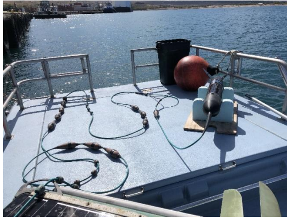
Figure 21. Tow Body and Tow Cable staged for launch aft of the Wave Glider.
