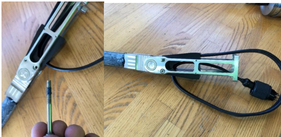
Figure 47. Apply Loctite 243 to the threads only where they will interface with the opposite bracket side (A). Use the two (2) screws to secure the two halves of the Tow Cable attachment brackets together.
