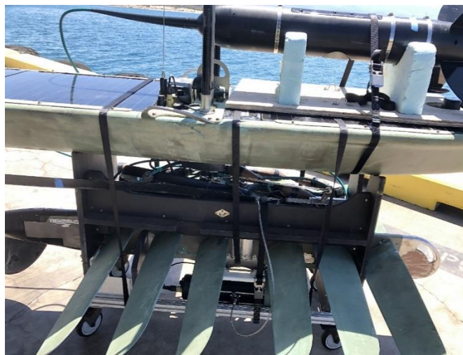
Figure 11. Wave Glider with Tow Body-equipped Winch bundled for loading and transport. Extra straps are used to secure the Winch housing to the cart frame (bottom), the Sinker to the stand, and Tow Body to the Float (top).
