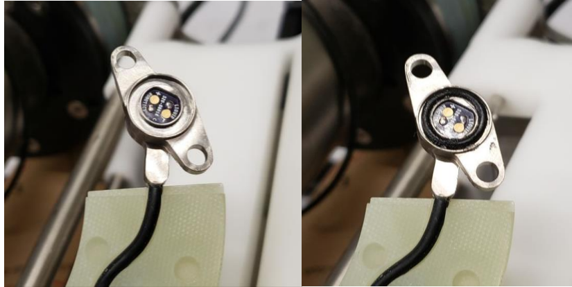
Figure 59. Clean the exposed 2-pin Thin Line Terminus a non-linting wipe (Kimwipe) and isopropyl alcohol. Place the lubricated O-ring in the groove on the Thin Line connector terminus(B).
