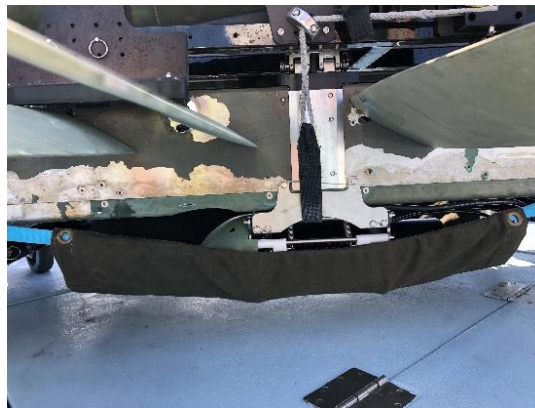
Figure 13. On Rapid Stands with Hammock installed, the Winch is supported and is ready for loading and transit.
