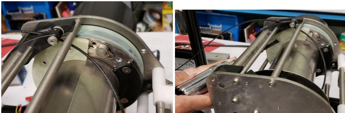
Figure 60. Route the Cable Clamp through the spool shroud and over the proper mounting holes (A). Loosely secure the Cable Clamp with 3x M5 flat head screws while making sure the Thin Line Terminus aligns properly. (B)
