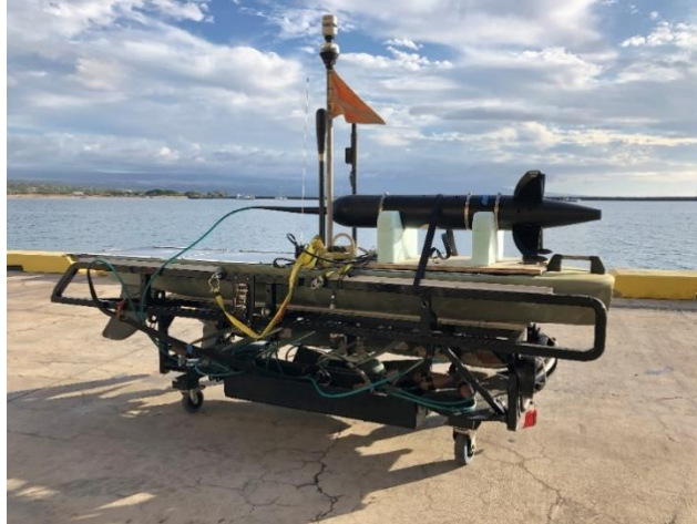
Figure 10. Wave Glider in Rapid Deployment Stand, configured with Winch and Tow Body, ready for hoisting and transit.
