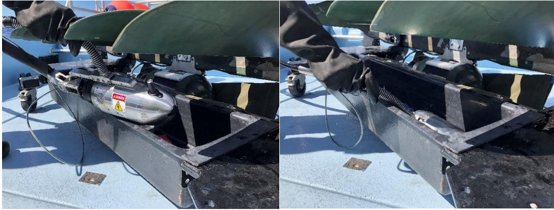
Figure 28. Sinker placed in the storage bin with the Snubber (spring section) pointed away from the Sub to protect the Thin Line interface. Make sure all of the Thin Line is in the storage box and not dragging on deck.
