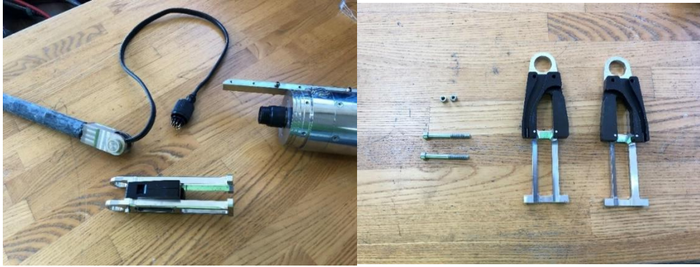
Figure 45. The tow cable attachment bracket removed from the Sinker (A) and separated (B).
