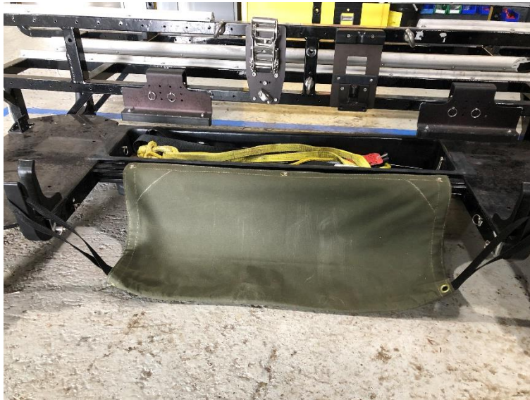
Figure 95. Tarpaulin with the strap loosened to allow access to a Winch mounted to a Sub.
