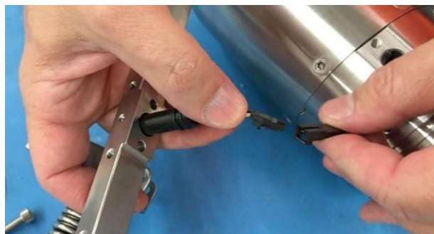
Figure 69. Disconnect the black connector between the Sinkers and the penetrator.
