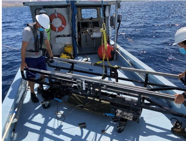
Figure 30. Saddle stacked on top of the Cart. The Sub Wings have been removed in this picture; this can be done later if deck space is not limited.
