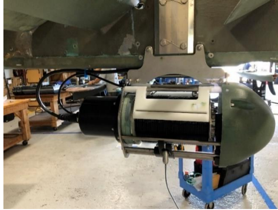
Figure 43. Winch-specific expansion cable arranged properly.
