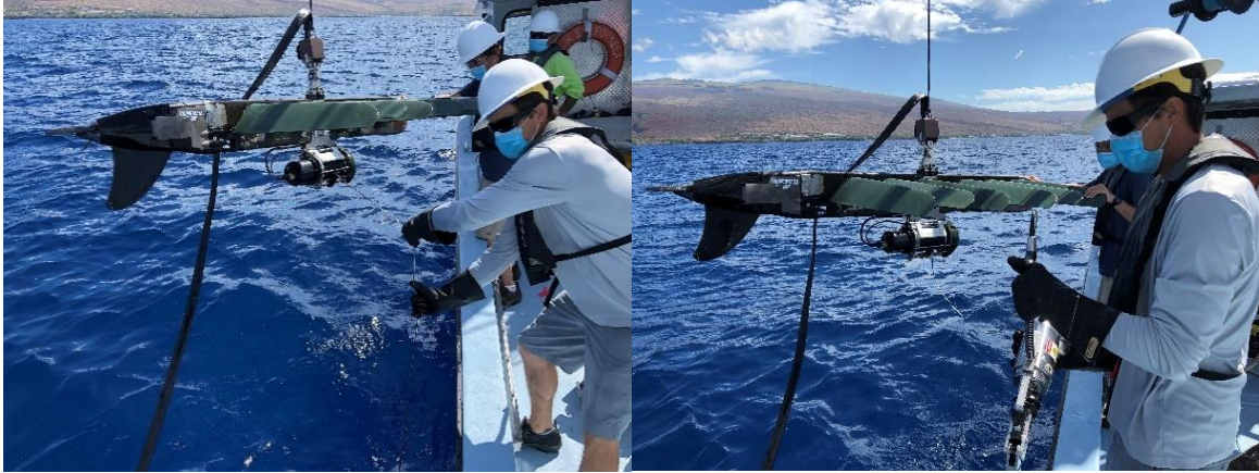
Figure 24. The Sinker crewmember should capture the Sinker by controlling the Thin Line using a boat pole or by hand (A, B, C). When grabbing and holding the Sinker, ensure the Thin Line does not contact any sharp or abrasive surfaces, and is not crushed, stepped on, or twisted. Carry the metal housing where possible.
