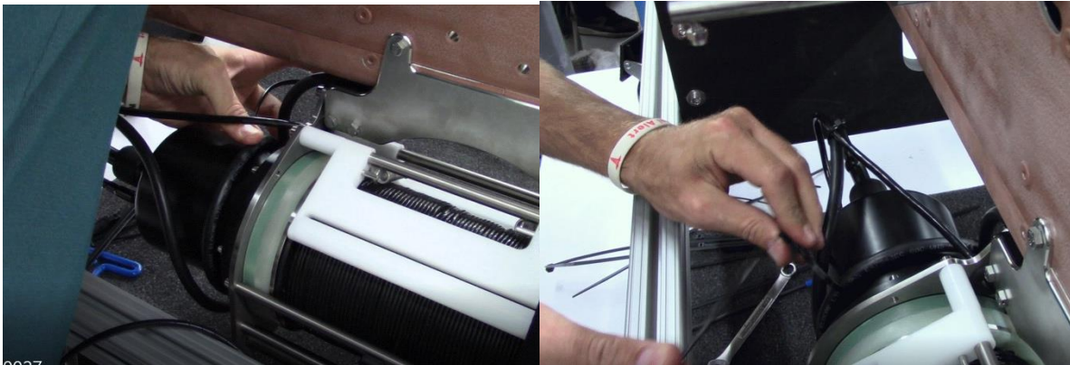
Figure 42. Swing the Winch left and right to the stops to make sure there is enough slack in the expansion cable.
