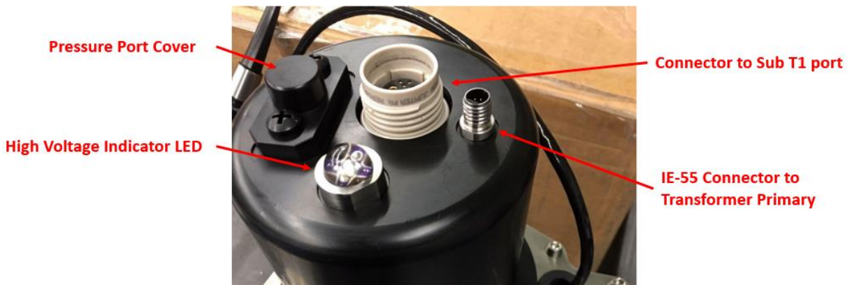
Figure 6. Annotation of the components at the aft of the Electronics Enclosure.
