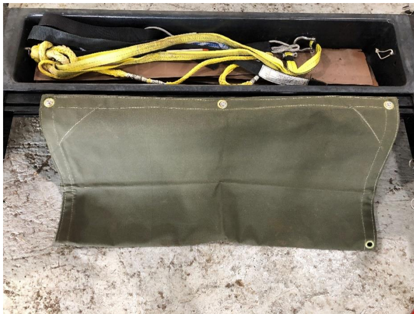
Figure 89. Tarpaulin folded in half and secured with 3x M6 screws.
