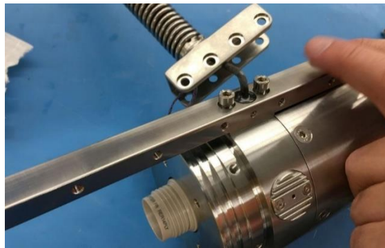
Figure 68. Remove the two socket head cap screws attaching the rail to the Sinkers.
