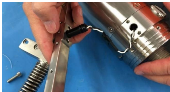
Figure 68. Remove the two socket head cap screws attaching the rail to the Sinkers.
