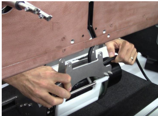
Figure 40. Align the Winch bracket with the threaded holes on the Sub. Route the Souriau expansion cable rearward in the plastic bearing.
