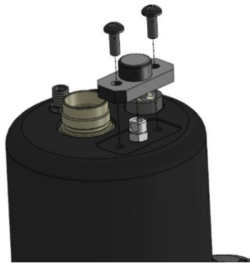
Figure 72. Exploded diagram of pressure port cover on Electronics Housing.
