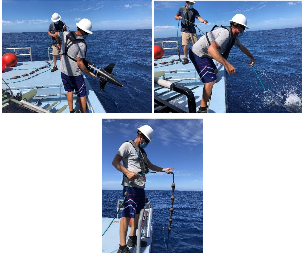
Figure 16. One crewmember should manage the Tow Cable while another manages the Tow Body or acoustic streamer (A). The Tow Body or acoustic streamer should enter the water first (B). Pay out the Tow Cable while taking care that the Tow Cable and towed payload do not come into contact with the boat or propellers (C).
