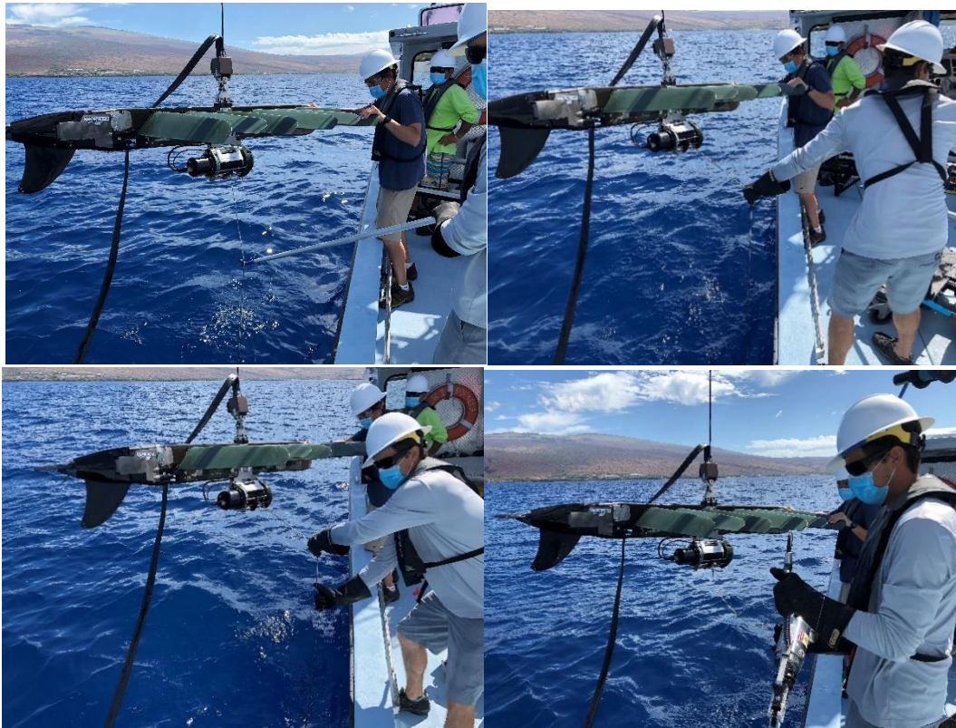
Figure 31. Figure 18. The Sinker crewmember should capture the Sinker by controlling the Thin Line using a boat pole or by hand (A, B, C). When grabbing and holding the Sinker, ensure the Thin Line does not contact any sharp or abrasive surfaces, and is not crushed, stepped on, or twisted. Carry the metal housing where possible.
