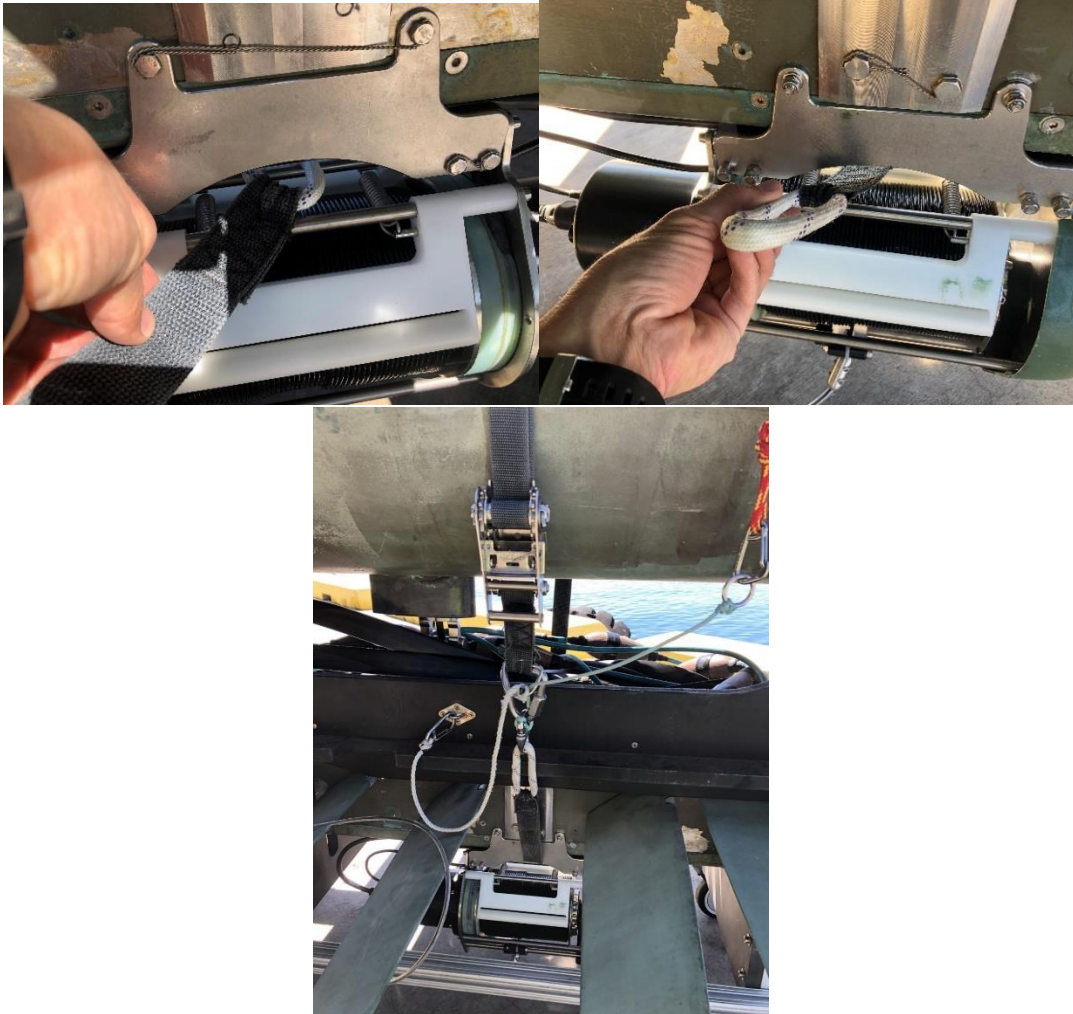
Figure 20. Route the Launch strap through the Winch Bracket (A & B), NOT through the metal rods at the top of the Winch.
