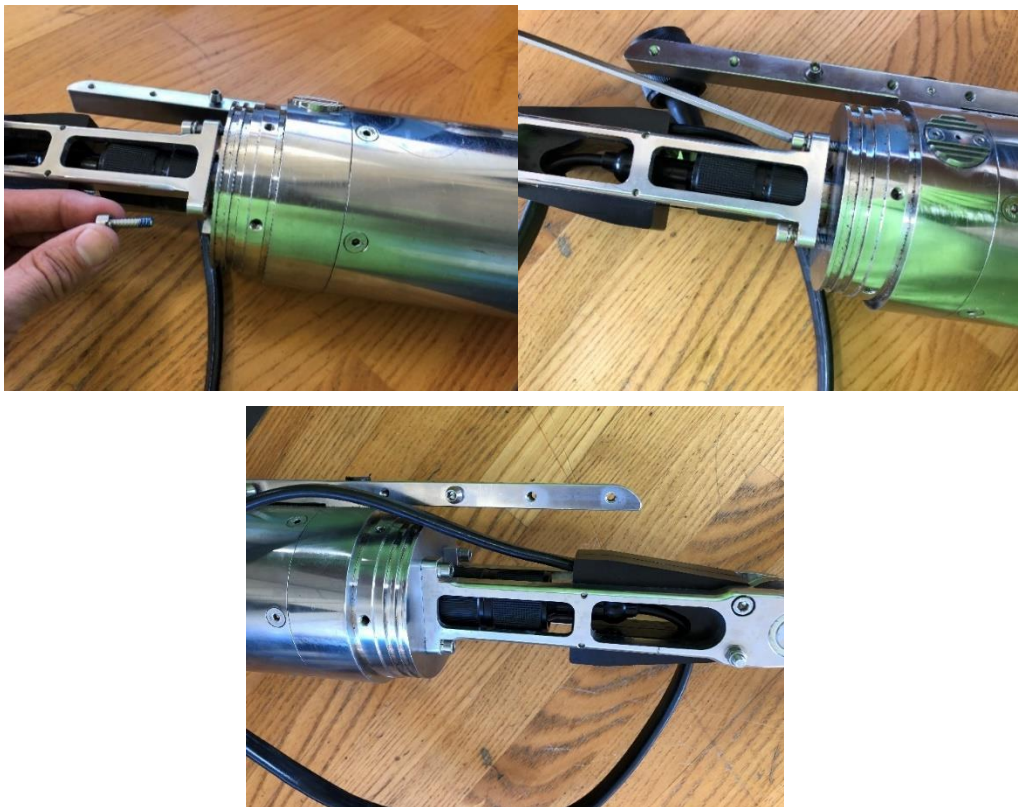
Figure 49. Secure the Tow Cable attachment brackets to the back of the Sinkers using 4x M5x18mm 316 stainless screws.
