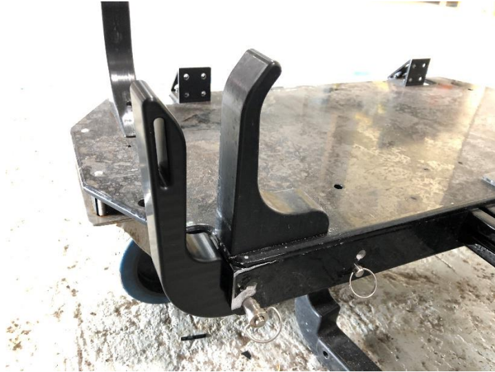
Figure 86. Front Sub Cradle configured for v200 and v300 sub (through lower alignment holes).
