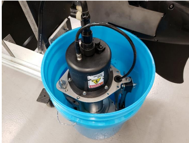
Figure 75. Winch in bucket filled with fresh water above the nearest silver end plate.
