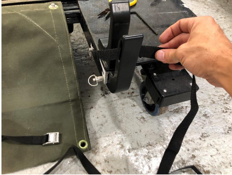
Figure 90. Strap threaded into the slot in the rear sub cradle.
