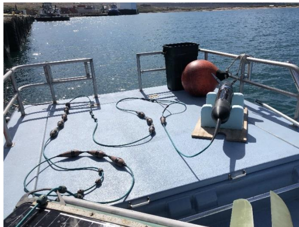
Figure 15. Tow Body and Tow Cable staged for launch aft of the Wave Glider.
