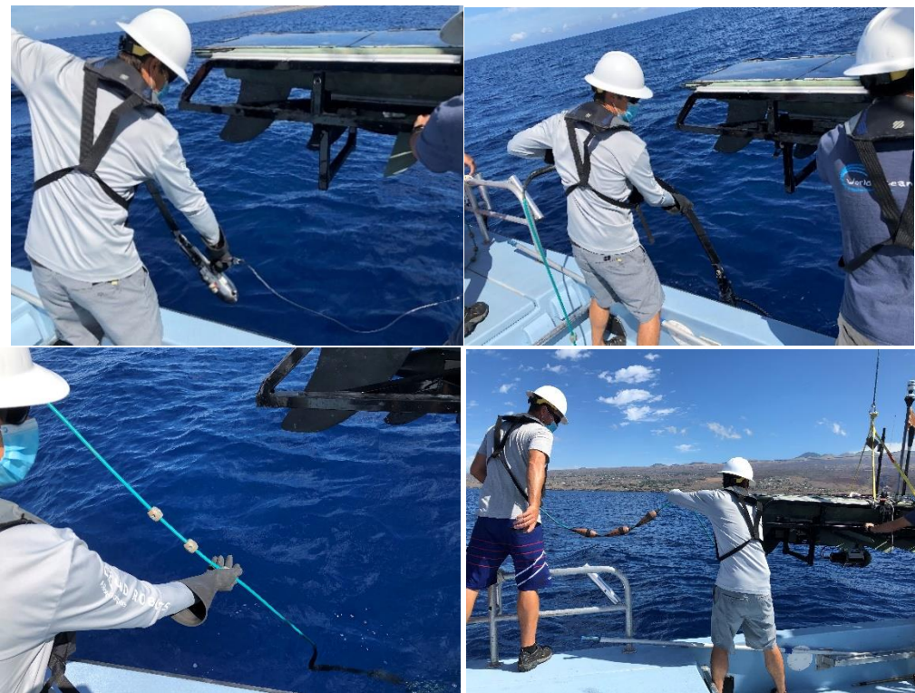
Figure 18. The Sinker should be placed over the freeboard and kept from free-falling into position (A). Lower the Sinker gently using the Tow Cable or drogue (whichever is directly attached to the Sinker) until it is fully
