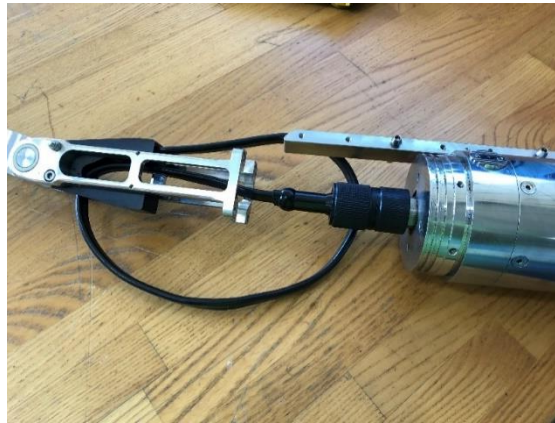
Figure 48. Tow Cable connected to the bulkhead on the back of the Sinkers. Route the ribbon cable as shown.
