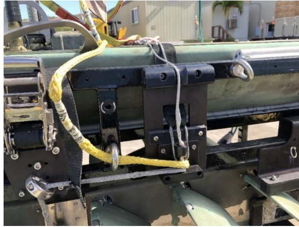
Figure 14. Properly routed Launch and Sub straps with safety pin in place.
