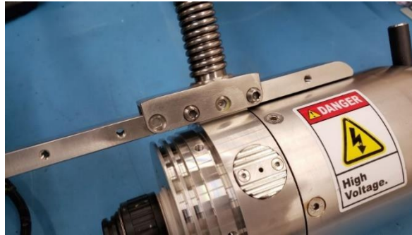
Figure 67. Remove the four screws attaching the Snubber to the Sinkers. There are two on each opposing side.
