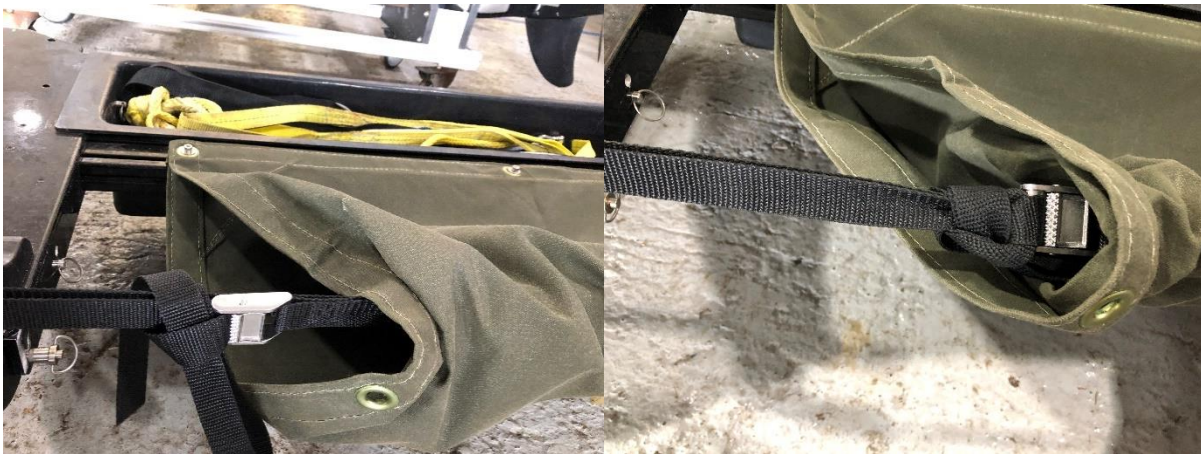
Figure 93. Overhand knot tied right against the strap cam to prevent it from loosening during use.
