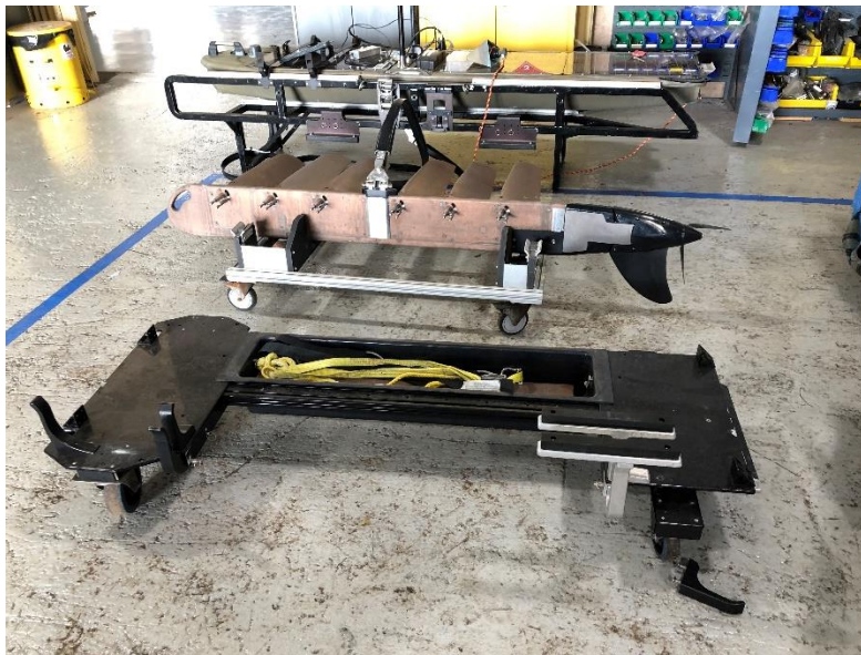
Figure 81. Rapid Stand with Wave Glider unstacked. Sub has been placed on a Legacy Stand cart.
