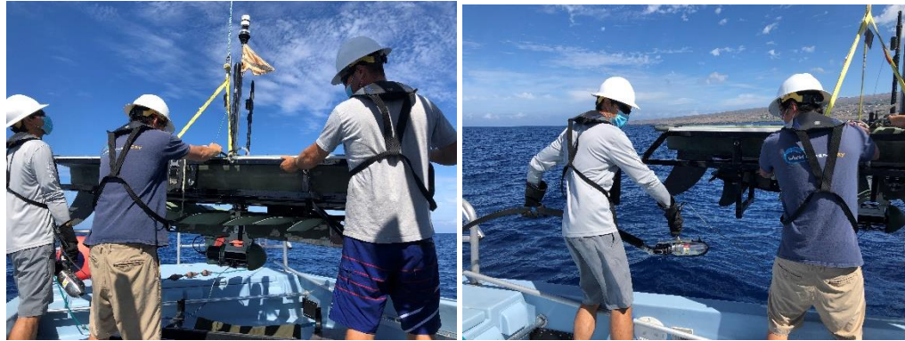
Figure 17. Wave Glider hoisted into position for launch (A). The Sinker crewmember follows the Wave Glider as it is hoisted and positioned over the freeboard (B).
