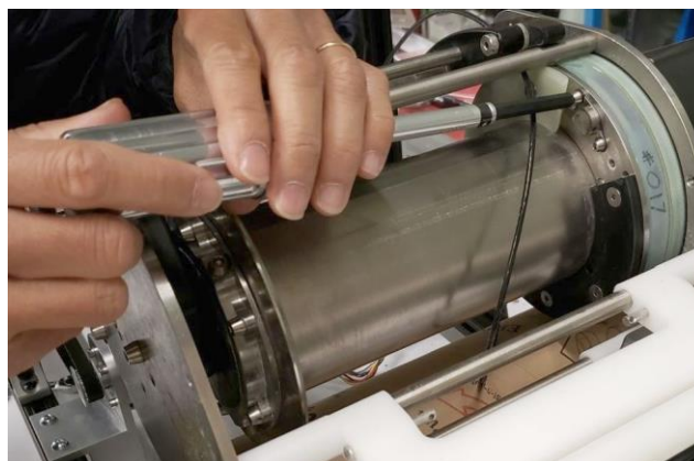
Figure 54. Remove the two M4 cap screws securing the Thin Line Terminus to the Secondary Transformer.
