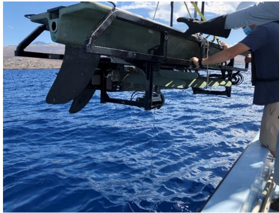
Figure 19. Wave Glider mid-launch, with the Sinkers and Tow Body deployed.
