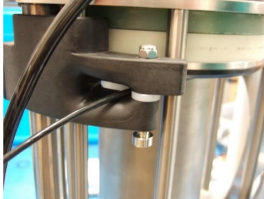
Figure 52. To remove the Thin Line from the level wind body (black), remove the shoulder screw, self locking nut, and nylon spacer. Slip the Thin Line out of the gap.
