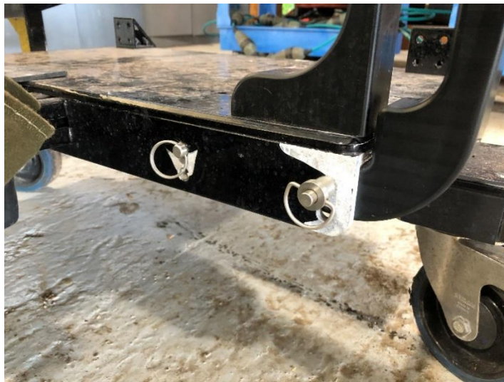
Figure 85. Rear Sub Cradle configured for v200 and v300 sub (through upper alignment holes).
