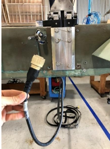
Figure 39. Souriau cable routed forward from the T1 port.
