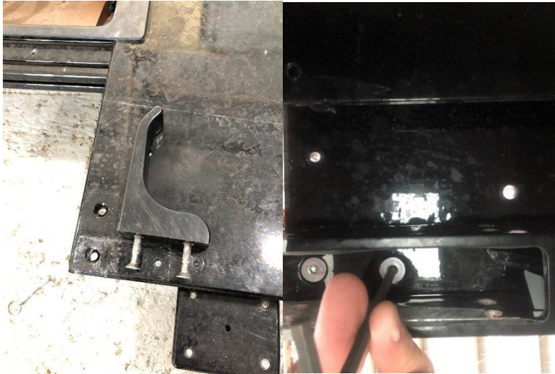
Figure 84. Mount the stock fixed sub cradle to the cart.
