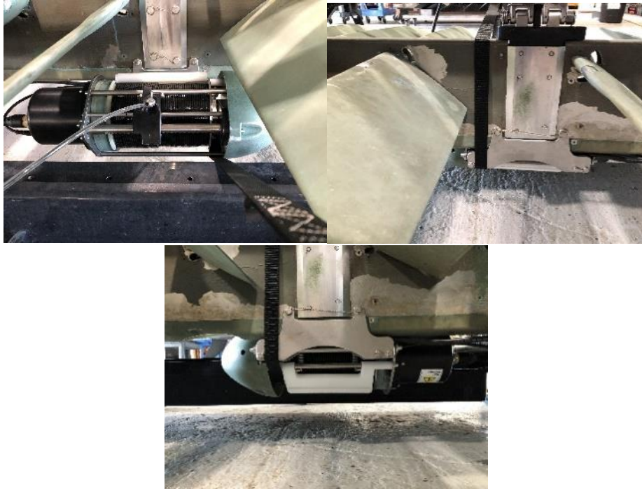
Figure 12. On Rapid Stands without Hammock installed, the Winch must be supported and secured by ratchet strap for loading and transit (A). The strap should wrap around the Sub (B) and support the Winch up to one side (C).
