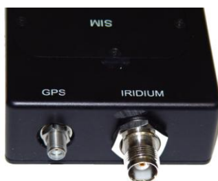
Figure 3. GPS Pass Through Connector Added on the A3LA-X Housing.
