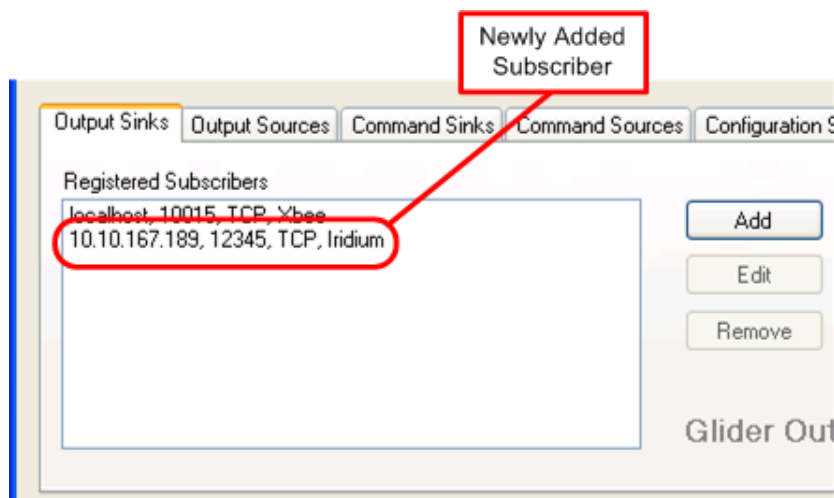
Figure 3-10: Packet Reflector UI Showing Added Output Sink
