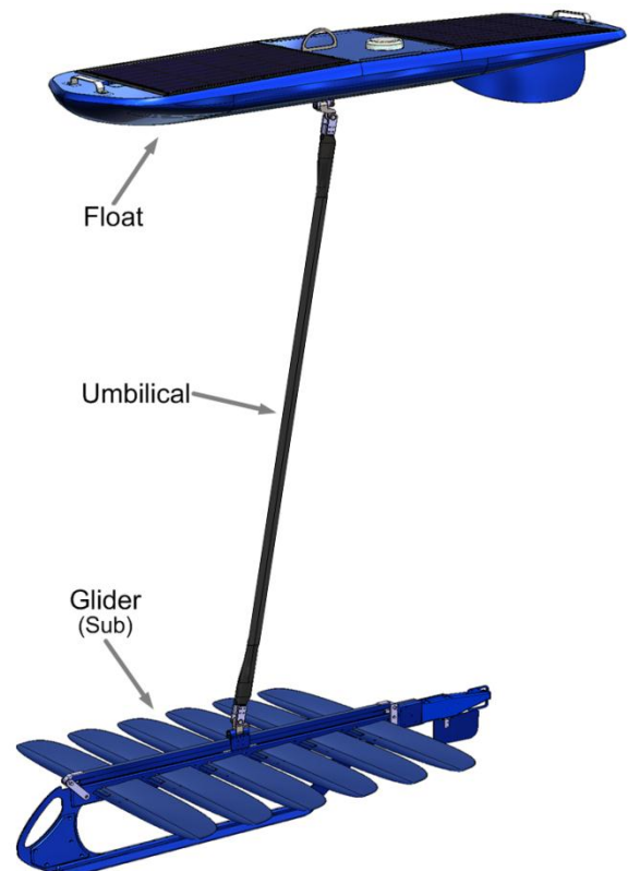
Figure 1-2: Wave Glider Vehicle Main Parts
