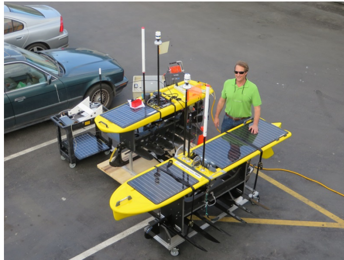
Figure 1. The SV3 Wave Glider is shown here beside the smaller SV2 Wave Glider.
