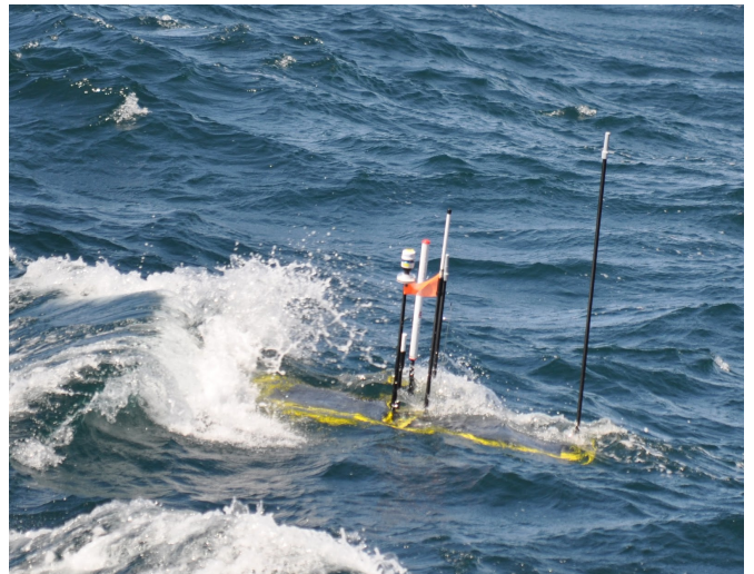
Fig. 1. The Wave Glider often gets pulled through the tops of waves by the driving foil, so the radio systems and antennas must withstand being completely submerged.
