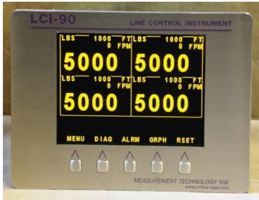
Figure 5.9 – LCI-90i Four Winch Mode
