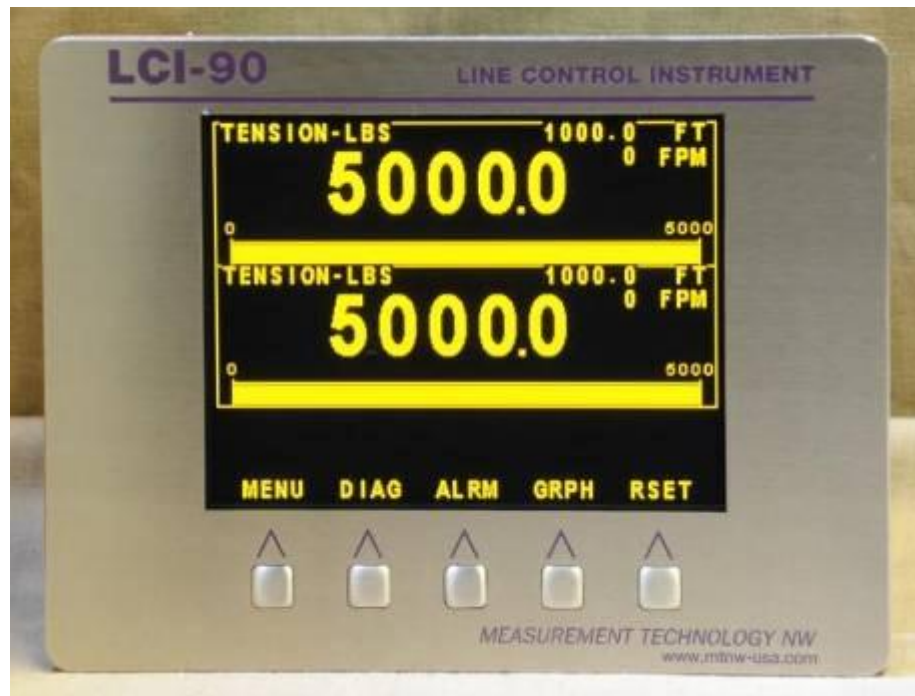
Figure 5.7 – LCI-90i Dual Winch Mode
