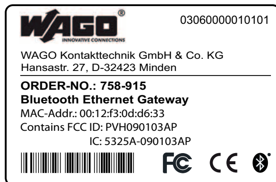
Figure 5: Nameplate on back/side
