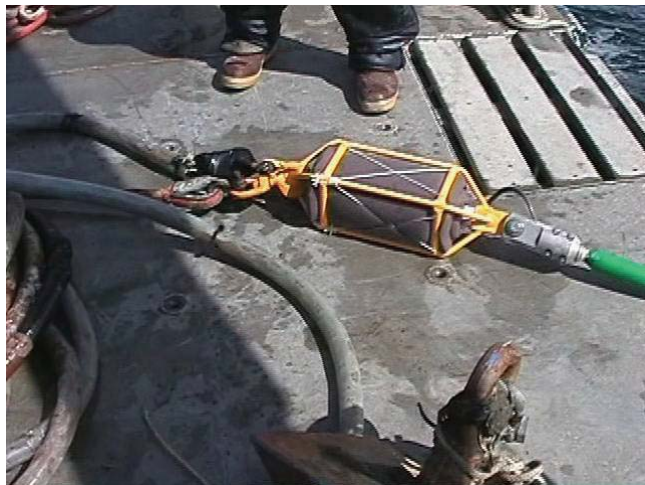
Figure 14: WELL1 Hydrophone wrapped in open-cell foam within the hydrophone cage, 19 March 2006.
