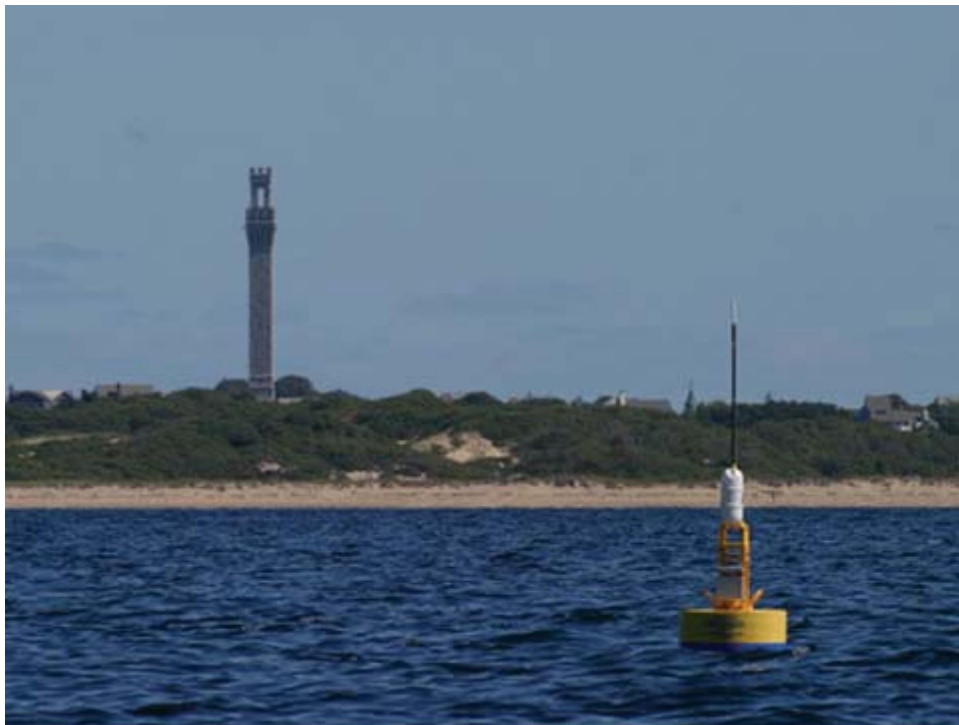
Figure 2: First AB deployment 14 September 2004, with surface buoy, electronics, radar reflector, and cell phone band antenna.
