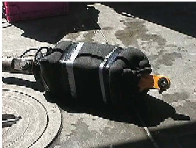
Figure 15: WELL2 entire hydrophone cage wrapped with open-cell foam, 19 March 2006.
