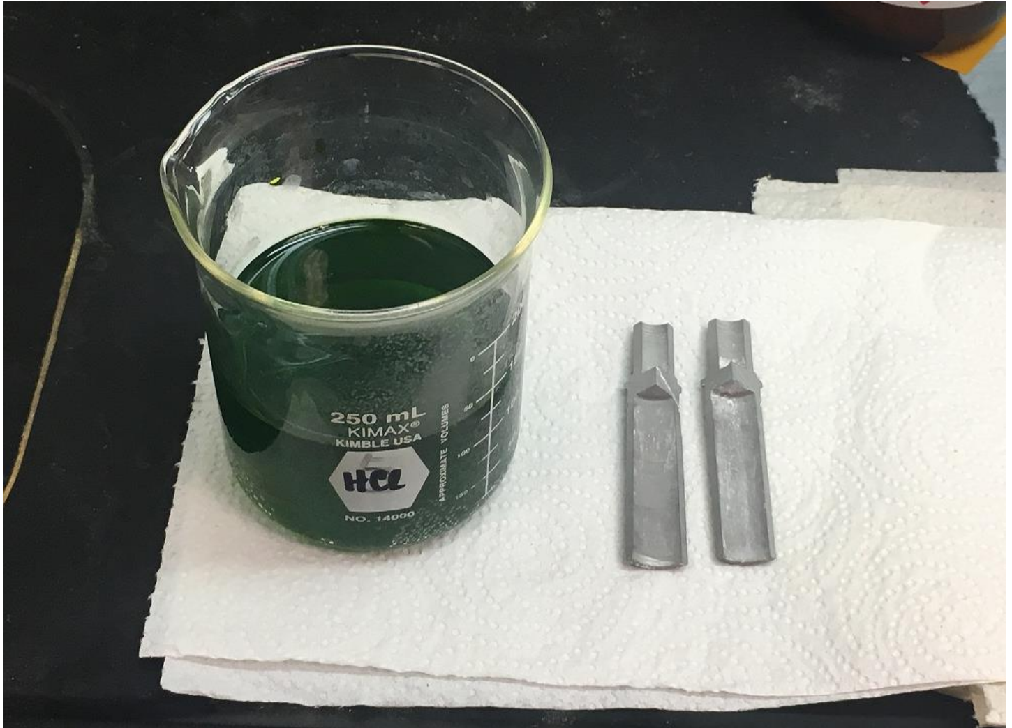
Fig 3. Samples #3 and 4#, application of etching finish by concentrated HCl acid overnight ~ 17 hours. One of samples was followed up with bead blasting on both sides and became sample #3
