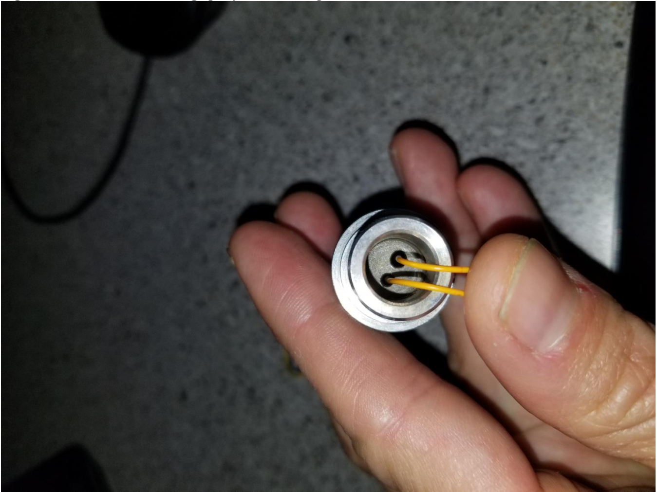
Figure 8: Reference to ensuring epoxy flows through 0.04" holes
