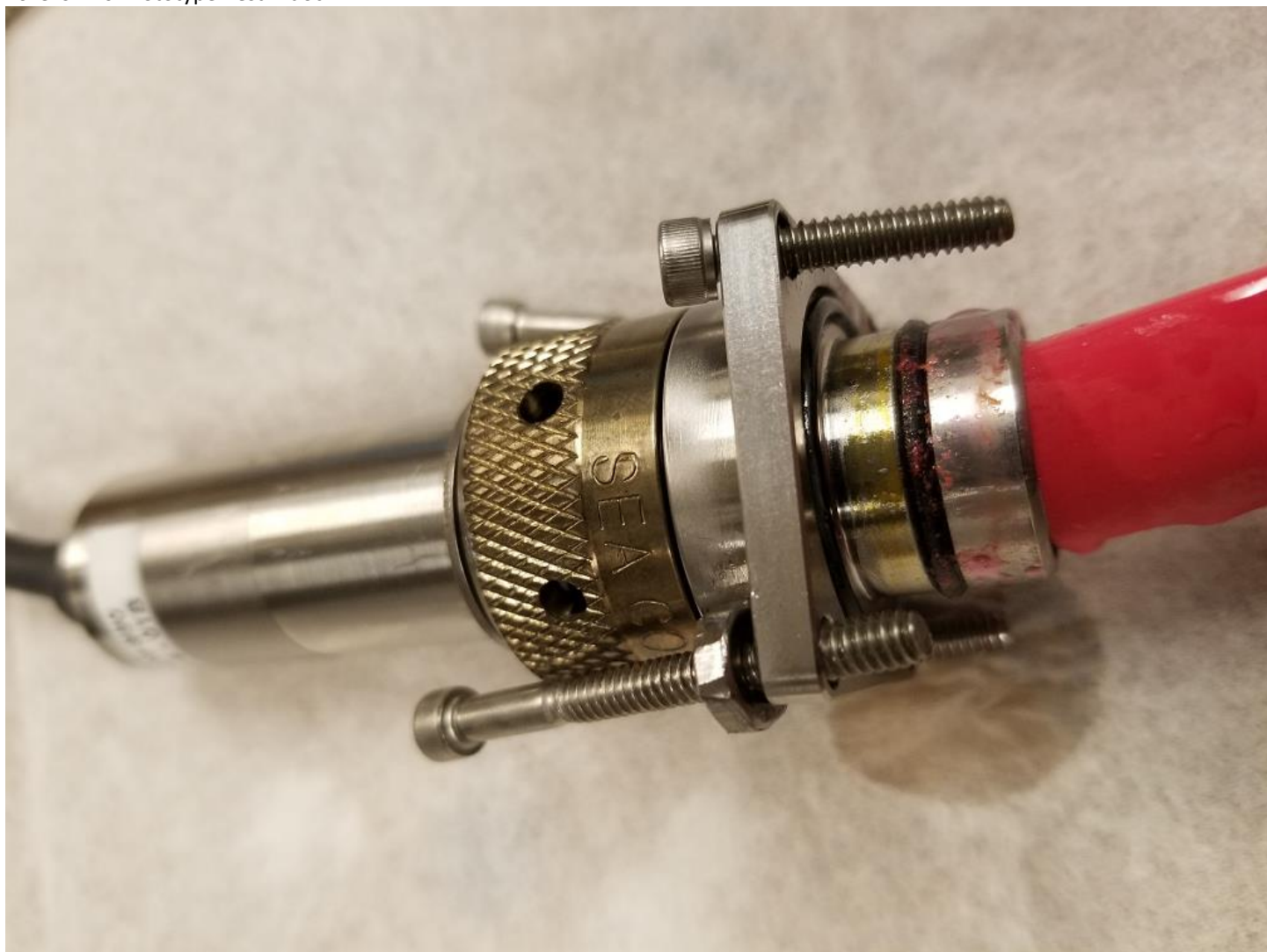
Fig 16. Assembly opened after pressure testing. Pressure relieve mechanism (4/15/2019, photo by Schnittger)
