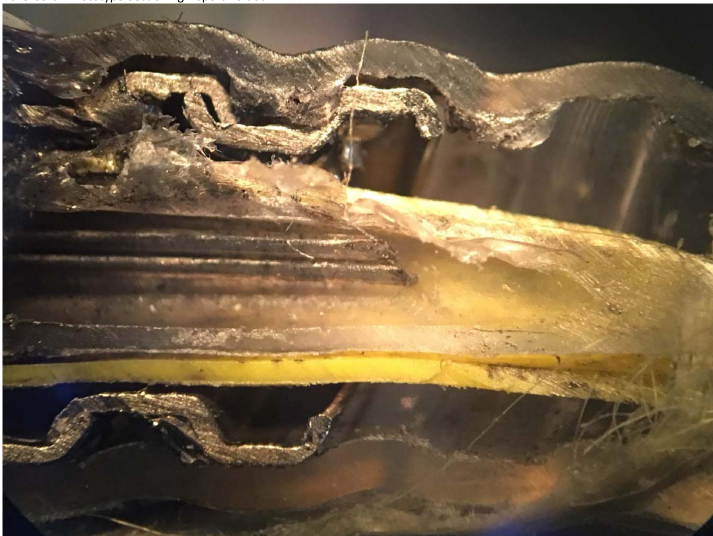
Fig 15. Close-up photo 5 of 5. Two optical fibers contained in one clear plastic tube
