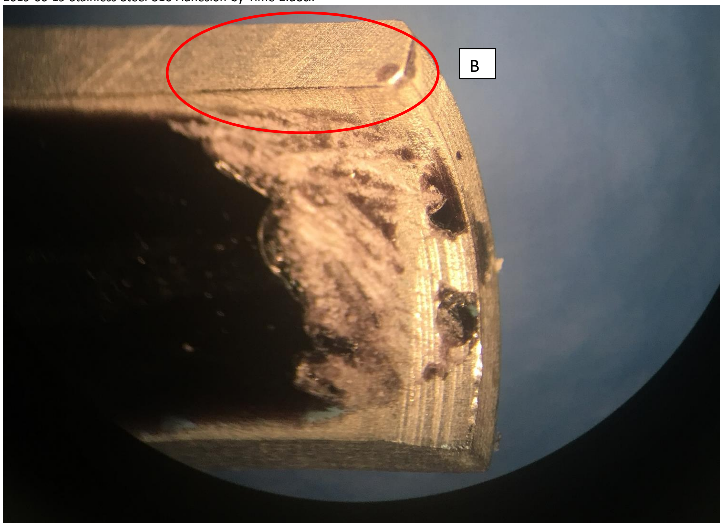
Fig 6. ~17 hours etched sample #4 from previous report. Area "B" is compared with 2 hours etching sample #5 (see Fig 7)
