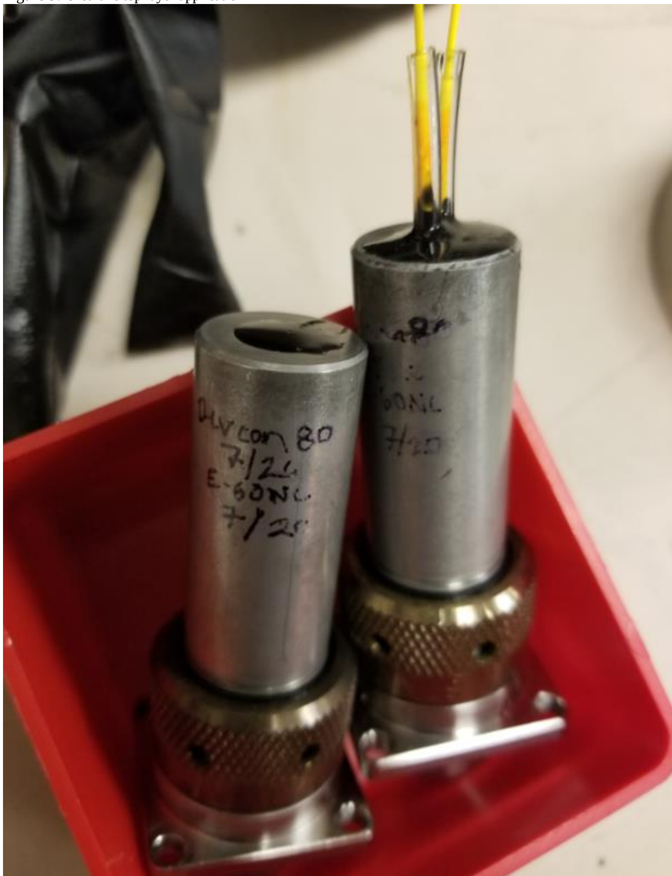
Figure 9: Urethane top layer application
