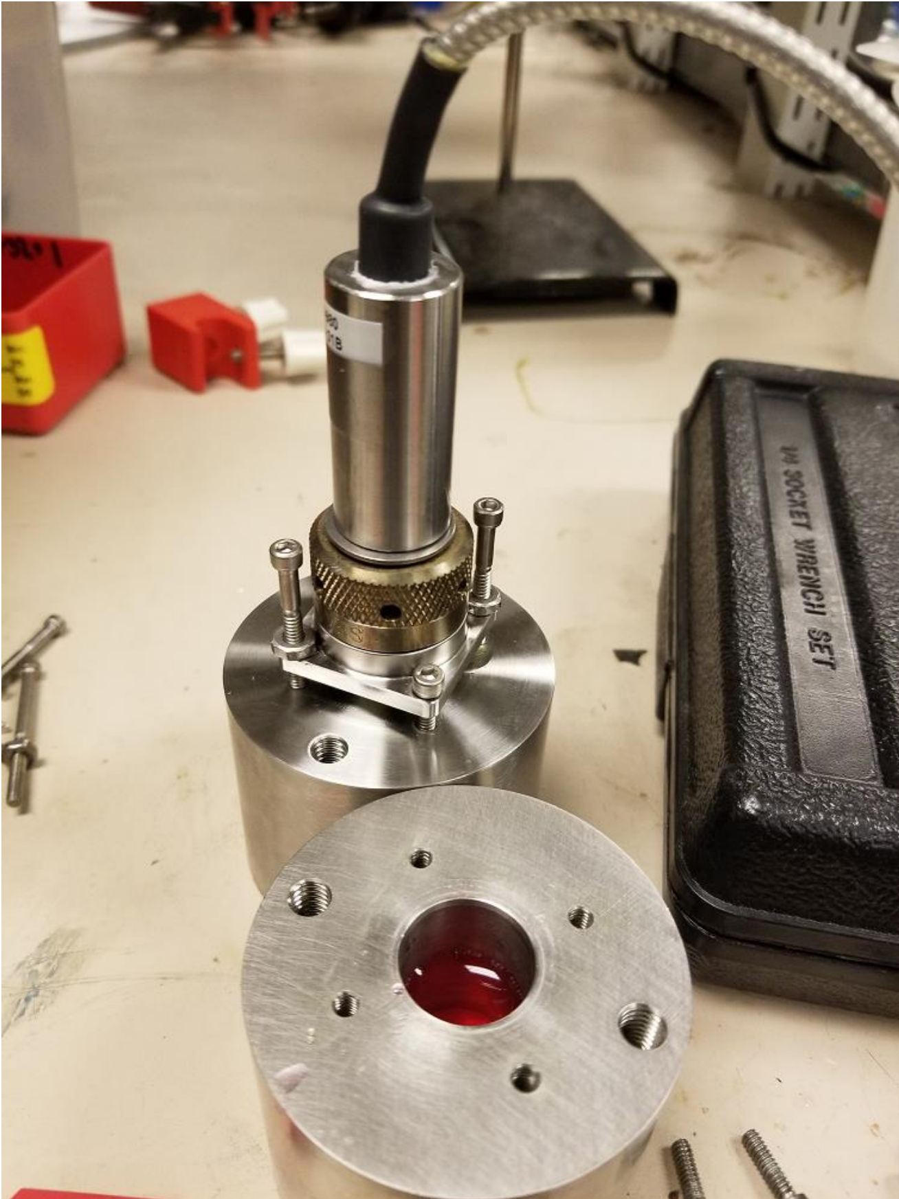
Fig 15. Assembly opened after pressure testing. Mixture of water with liquid-detecting dye is visible (4/15/2019, photo by Schnittger)
