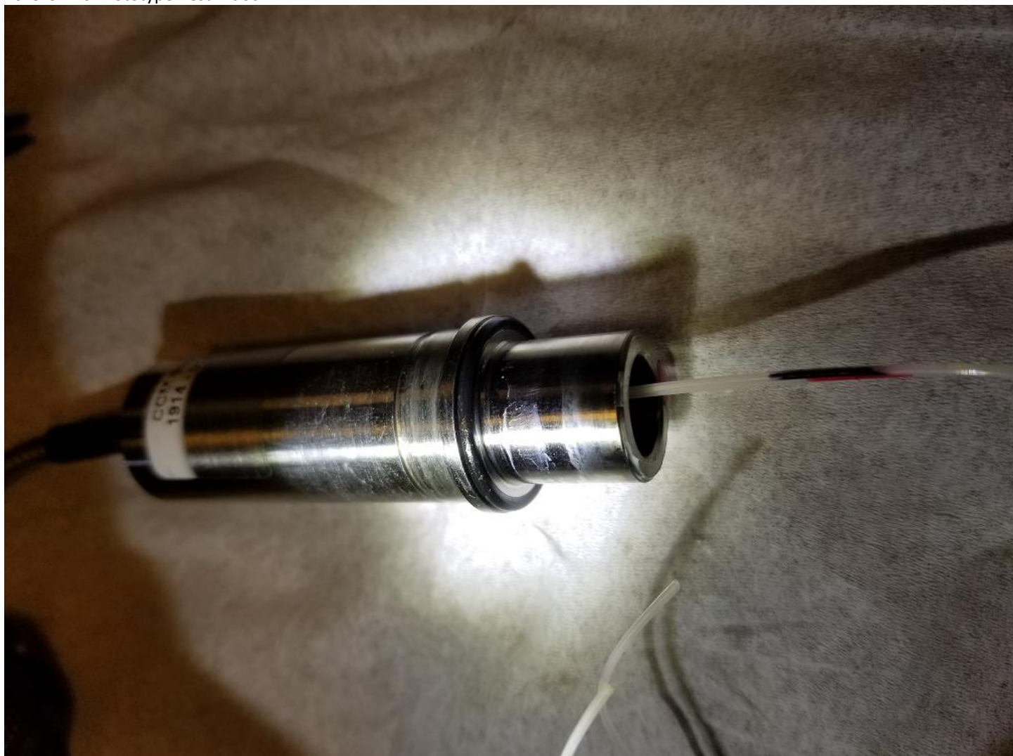
Fig 17. Assembly opened after pressure testing. Penetrator photo (4/15/2019, photo by Schnittger)
