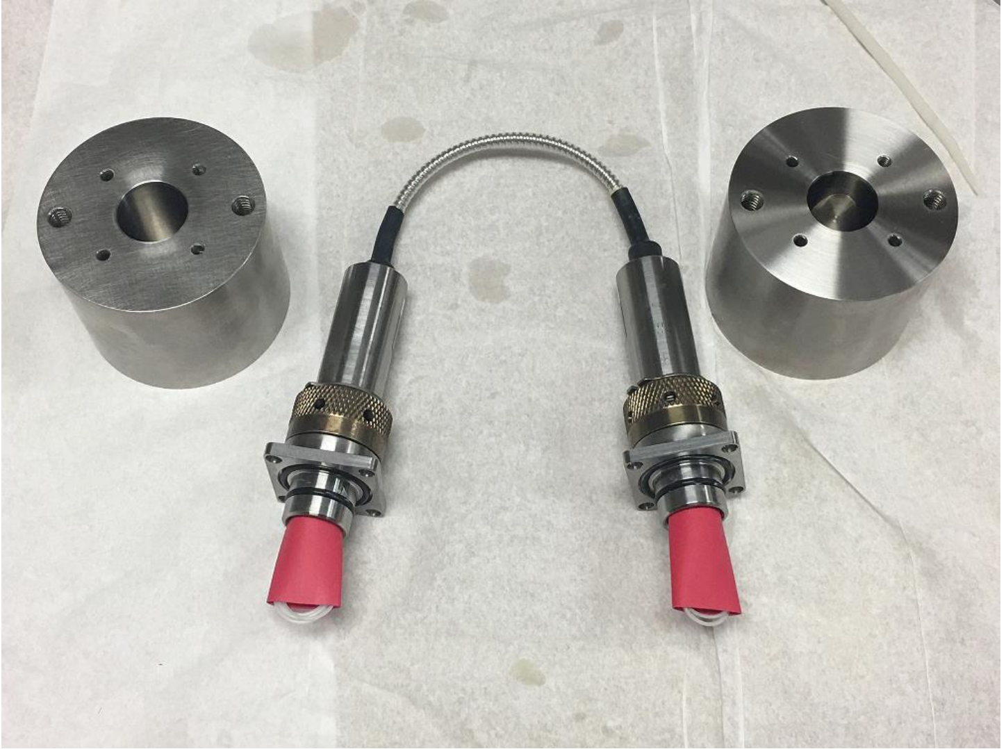
Fig 8. Assembly before pressure testing. Both fibers were trimmed to 7.5" length, and folded into about 0.75" wide x 1.5" long envelopes held with heat shrink tubing (4/10/2019).
