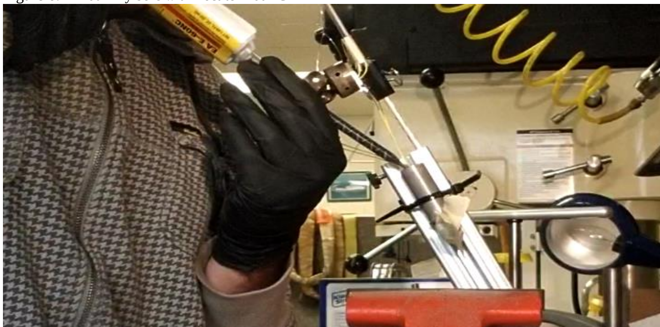
Figure 6: Fill dummy bore with Loctite E-60NC
