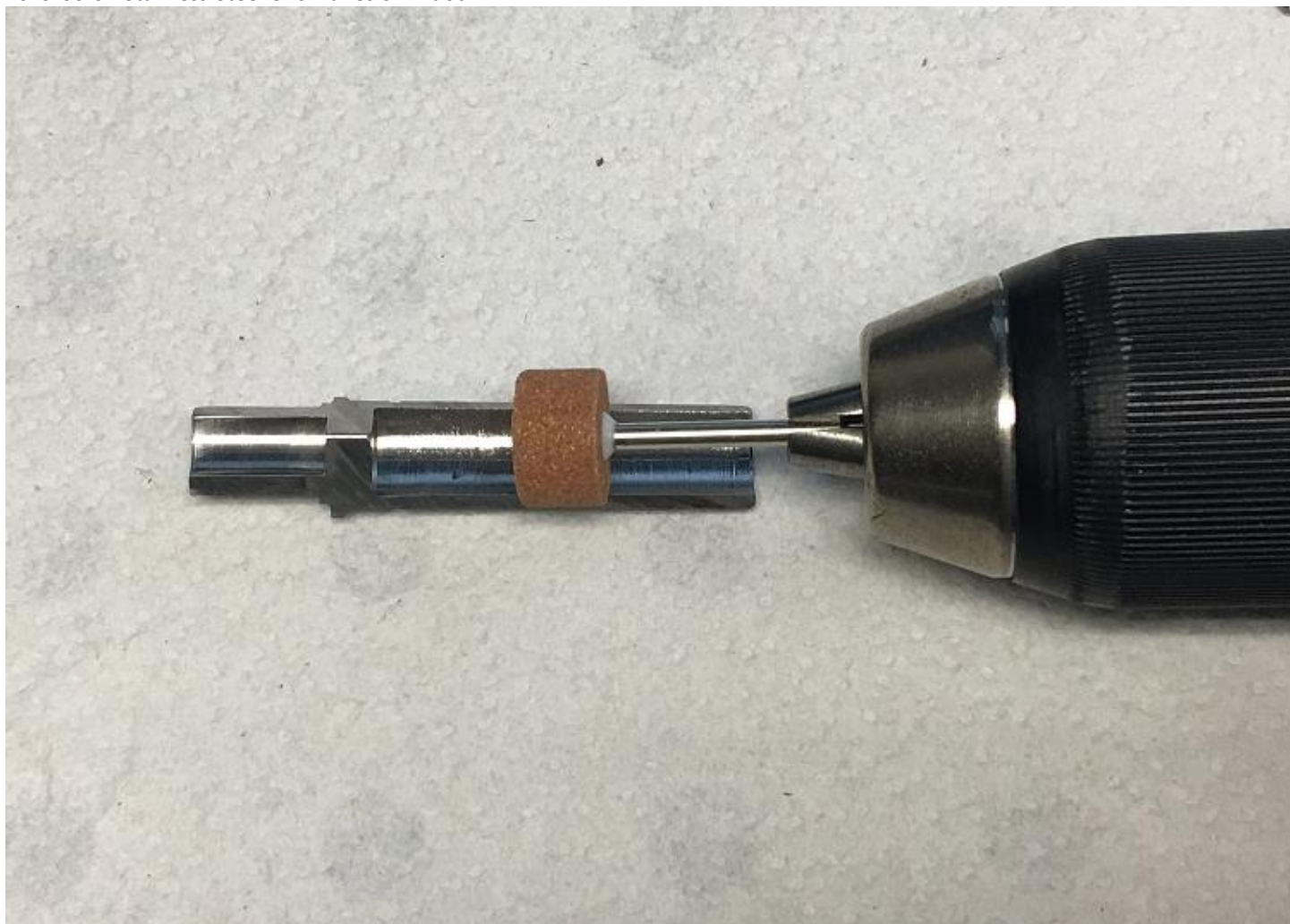
Fig 2. Sample #2, application of honing finish
