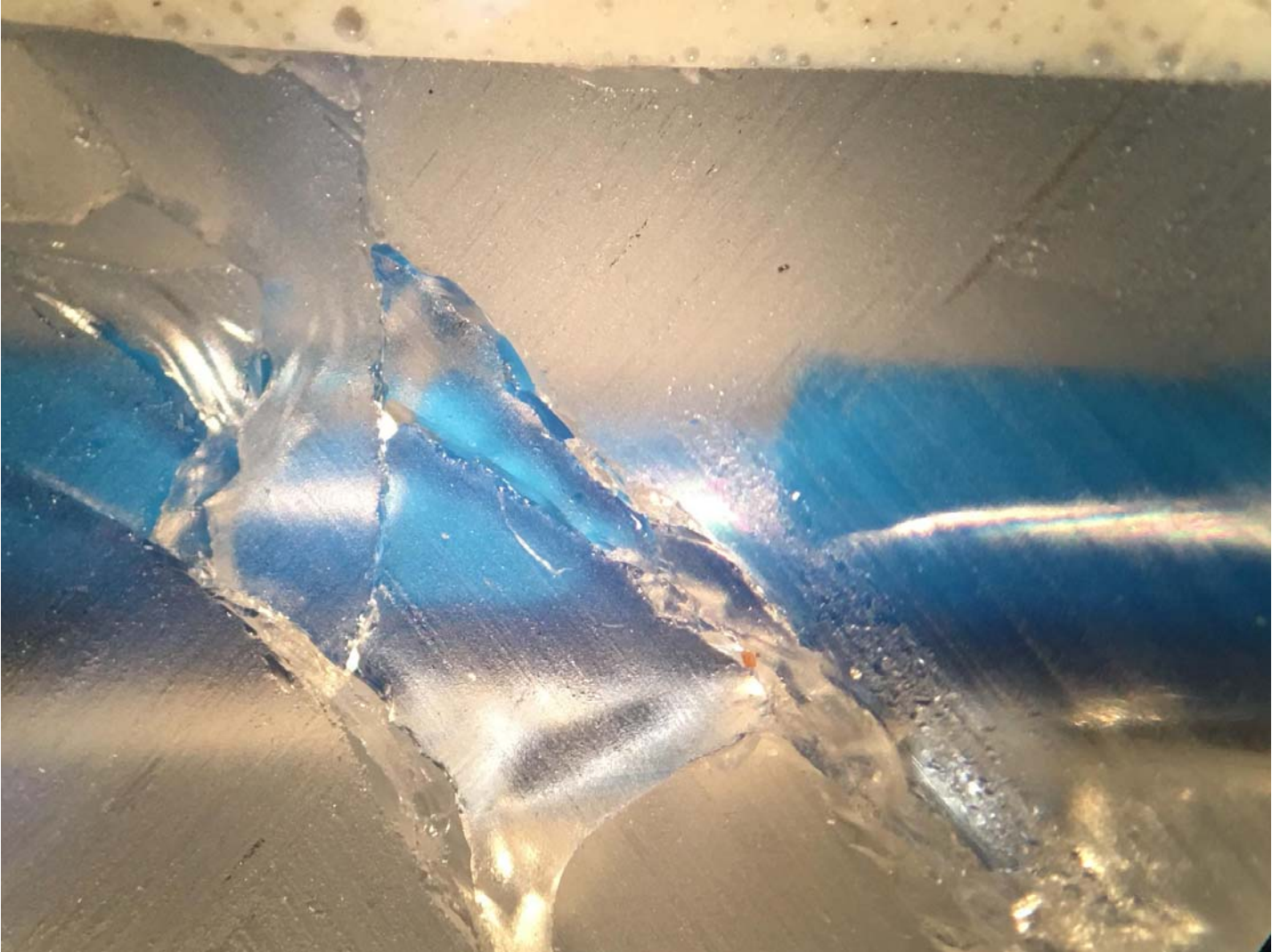
Fig 13. Close-up photo 3 of 5. Diagonal faults area in the middle of glass tube, suggesting possible fracturing under axial load (observation by Jon Erickson)
