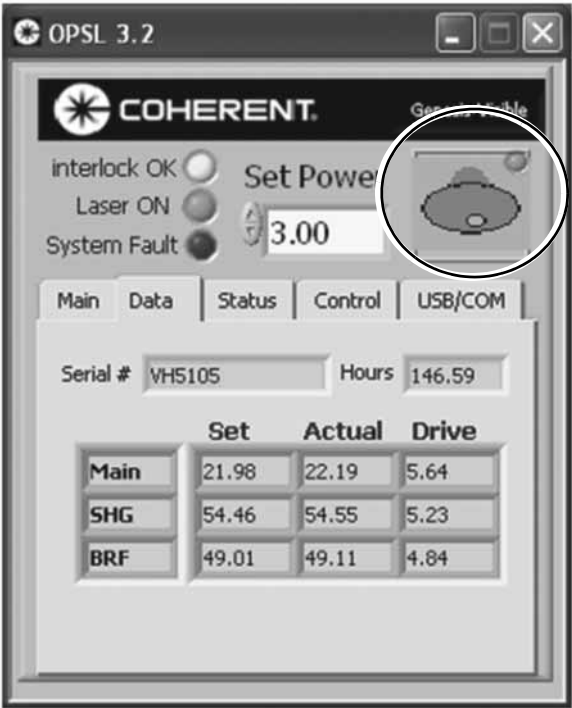
DATA: PARAMETER VALUES FOR SERIAL NUMBER, HOURS OF OPERATION, SET POINT AND ACTUAL TEMPERATURES AND DRIVE VOLTAGE ARE SHOWN. NOTE KEY POSITION IS ON.
