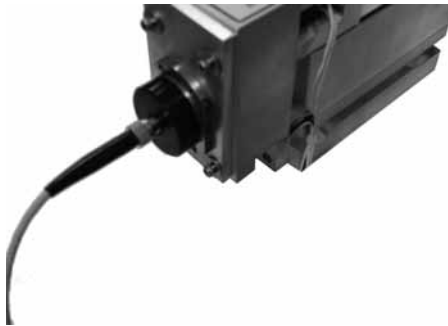
Figure 3-21. Fiber Connected to Port
